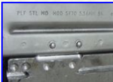
Alignment of plate anvil to rivets
