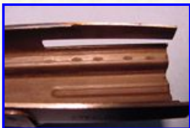
Spotwelds on dustcover, inside view.
