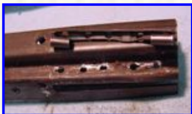
I ended up with a twisted and distorted bracket. This added considerably to assembly time as I reshaped it.
