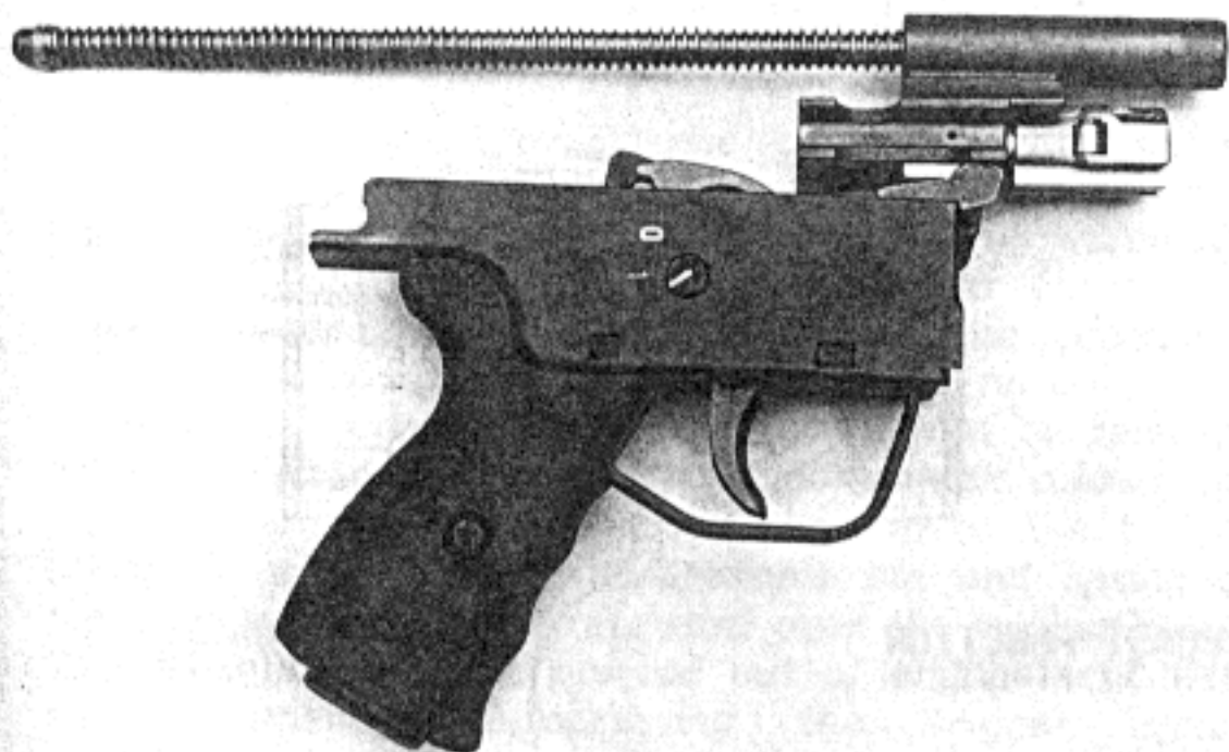
A right view of the modified Trigger and Grip Assembly, showing the relative position of the Release Lever and Tripping Block at a point where both are in contact. Fig. 20
