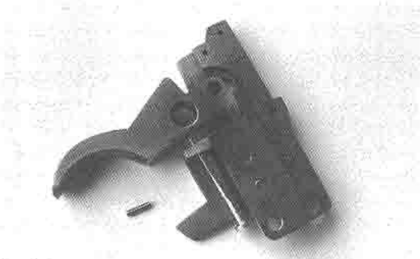
View showing the proper assembly of the sear/trigger spring rod. In this view, the spring rod (without the spring in place) is inserted into the oblong slot of the bent part of the sear, then into the other oblong slot on the front face of the trigger. The end of the rod has a hole into which a small pin is inserted to retain the spring assembly in place.
