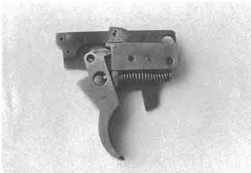
A right side view of the conversion trigger mechanism fully assembled as one unit.
