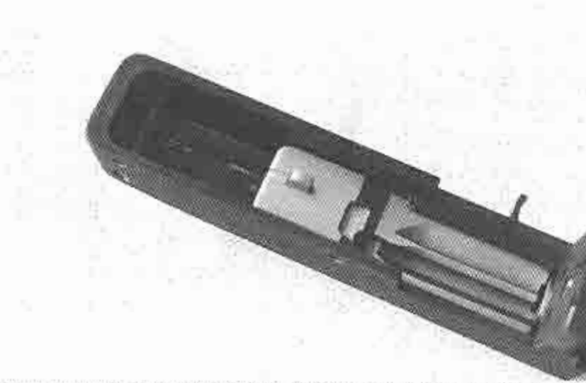
View showing the bolt mechanism fully assembled inside the receiver housing. In this view, the pivoting hammer design used for selective-fire is installed, and the hammer's lower part protrudes underneath the bolt rear end. The lower protrusion of the hammer in the underside of the bolt will hit the ignition shoulder (ejector pin) during bolt closure to fire the weapon.
