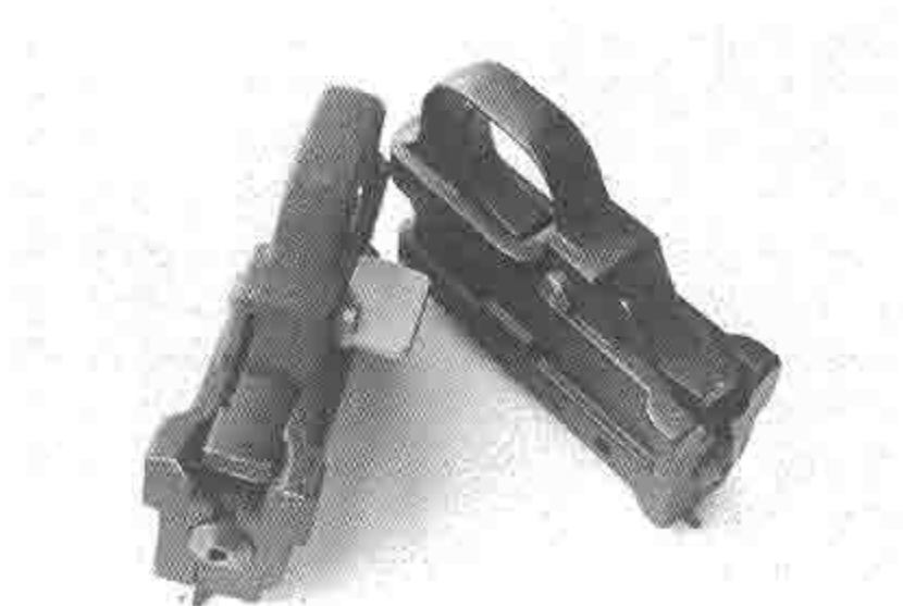
Bottom view showing the trigger housing assembly of the push-button-type safety of the factory (right) and the easily manipulated selector-lever-type of the converted model (left).
