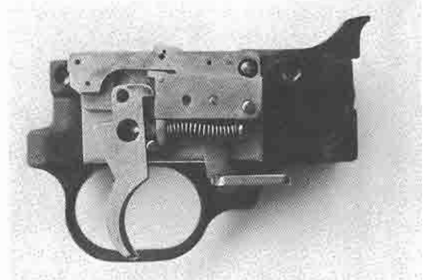
A detailed view showing the conversion mechanism outside the trigger housing frame. Assemble the mechanism while you are fitting the parts so you can see their proper relationship.
