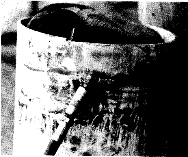
A hand grease gun is used to apply common lube grease to the end of an eight-inch cache tube prior to placement of the end cap.
