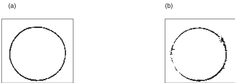
Figure 2.15 Acquired images of two different bottles. (a) Image of the mouth of a new bottle. (b) Image of the mouth of an older bottle with clearly visible intrusions
