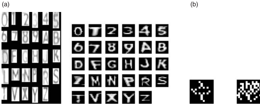
Figure 6.6 Character classification for license plate recognition. (a) Character sets from license plates, before and after normalization. (b) Selected features. The number of features is 18 and 50 respectively
