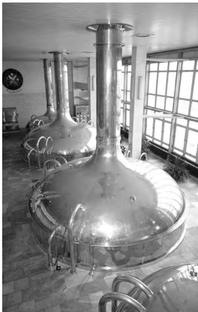
Large vats in which the fermentation process in the brewing of beer occurs.
