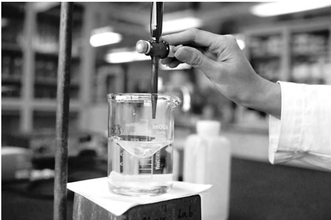
Titration burettes are used to carefully control the pH of solutions used in laboratory procedures.
