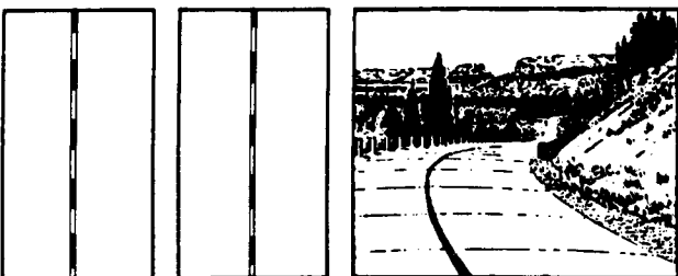
Figure 105. Hard-Surface, Medium-Duty Road. LARGE-SCALE: Two or three lanes wide. Unless otherwise labeled, the road is two lanes wide. MEDIUM-SCALE: Two lanes wide.
