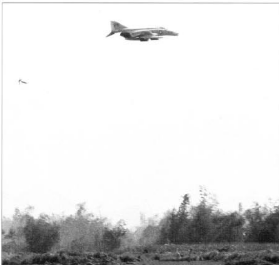
'Snake-and-nape', high explosive and fire bombs, are delivered by an F4 Phantom dropping a 500 pound MK82 Snakeeye bomb on Communist trenches in the tree line. The fins of the bomb open to delay its flight until the aircraft is clear of fragments. At this point the infantry would also hit the deck. (USNI)
