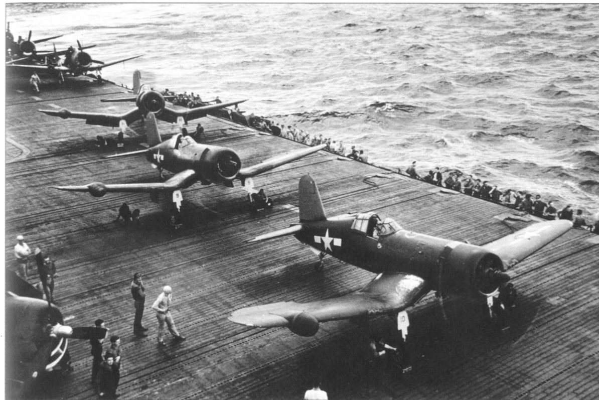
As the war progressed the need for night fighters became more and more important. These F4U-2s have been equipped with Army-Navy standard alternating pulse radar AN/APS-4 mounted on the right wing. They are flying from the USS Intrepid CV 11 in February 1944. (National Archives)
