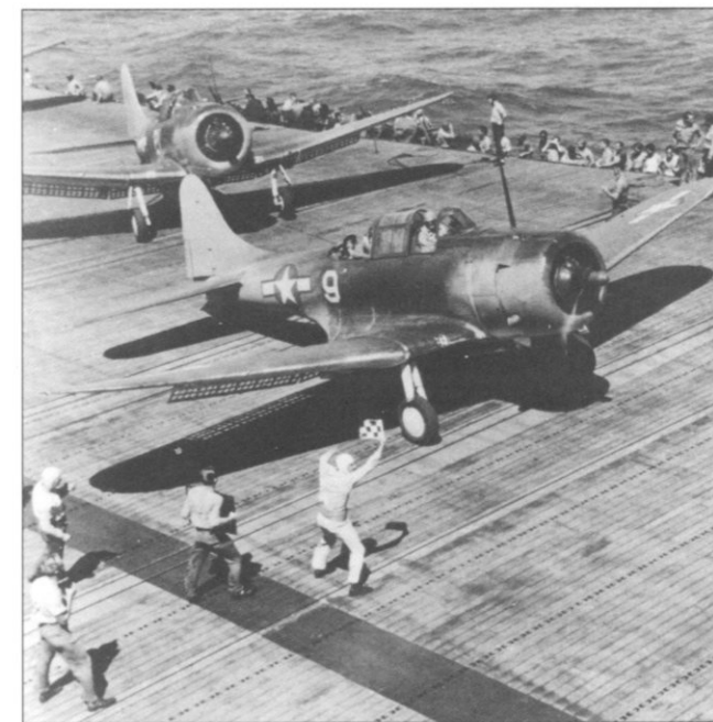
The SBD-5 in this 1944 photograph is on final full power prior to launch. The pilot has his eyes fixed on the aircraft handler and his checkered flag. When the handler drops the flag the pilot will release his brakes and launch the plane. (National Archives)
