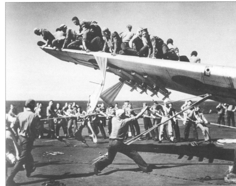
The US Navy continued to experiment with air-launched rockets throughout the war. Shown here mounted on the wing rails of a TBM "Avenger" are the 3.5 in. ARs. In this photograph Navy deck crew attempt to keep the TBM from going over the side of the ship. (National Archives)
