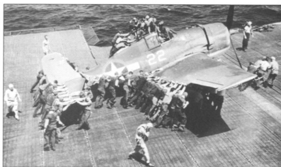
Plane crews had to move quickly to re-spot aircraft forward on the flight deck following a landing (1943). (National Archives)
