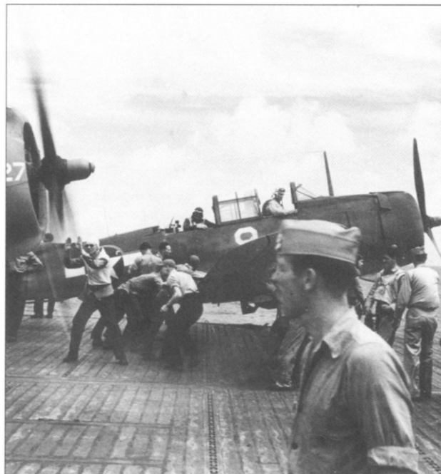
The organized chaos of spotting planes for launch is clearly illustrated in this photograph. All crew members had to be constantly aware of the dangers of whirling propellers. (National Archives)
