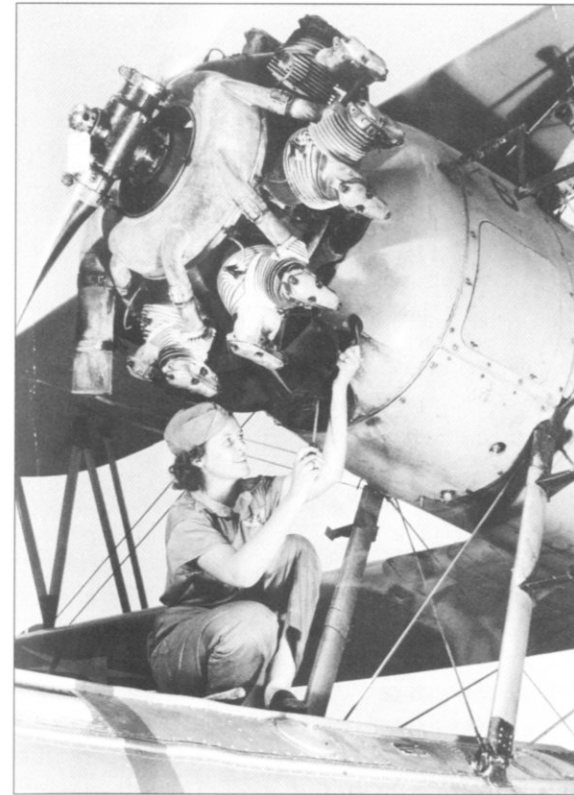
As the need for pilots grew so did the need for aviation mechanics. This USN WAVE (US Navy woman mechanic) works on the radial engine of one of the training command's "Yellow Peril" floatplanes c.1942-43 (National Archives)
