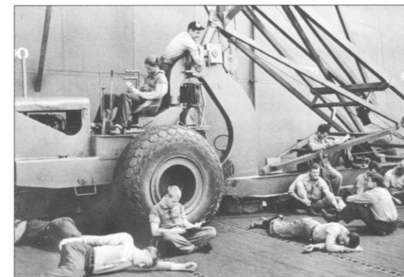
One important piece of equipment for dealing with damaged aircraft on a flight deck of the carrier was this motorized crane, known as "Annie" to the crew. The crane replaced smaller tractors that had hitherto been used for aircraft removal. (National Archives)
