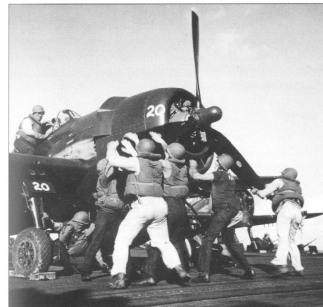
American naval aircraft such as this F6F Hellcat were of a radial engine design, which necessitated manual turning of the prop prior to starting the engine of the aircraft. (National Archives)
