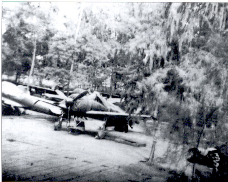
Type 0 Carrier Fighters (A6M) in the dispersal area surrounded by jungle at Buin on Bougainville. Note the Japanese-style steel matting on the ground. (USAF photograph)
