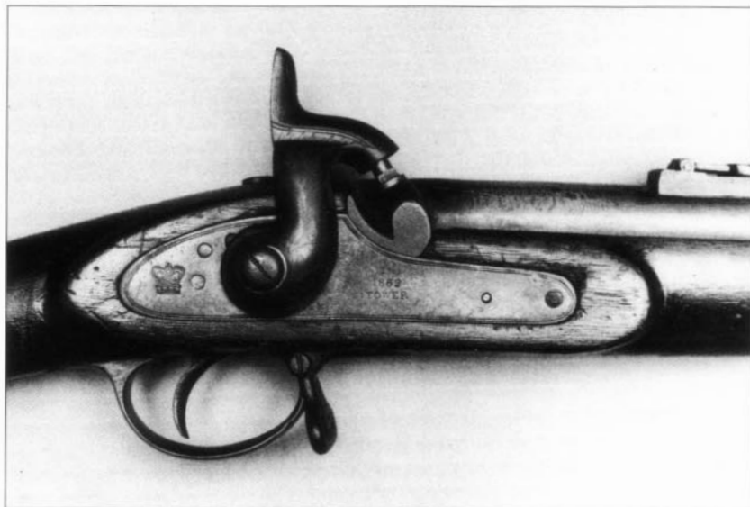
A detail of the lock plate of a P1858 Enfield-style rifled musket made under contract for American Civil War forces. (Author's collection)
