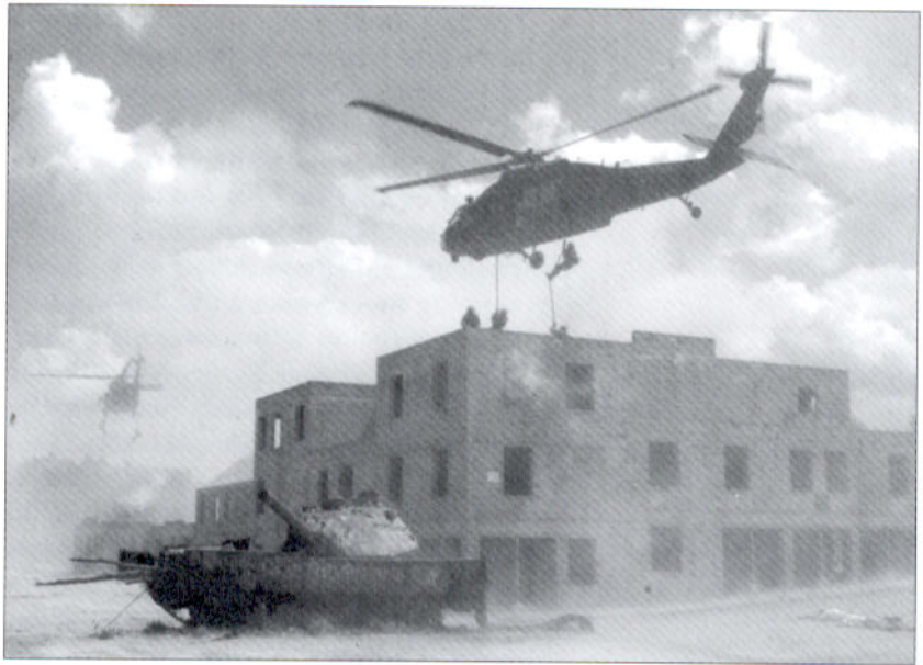
Rangers fast roping from Black Hawk helicopters onto the rooftops of a mock city. One problem with fast roping is that in dry terrain the rotor wash will kick up tremendous amounts of dirt causing "brown-outs." (Nancy Fisher, USASOC)
