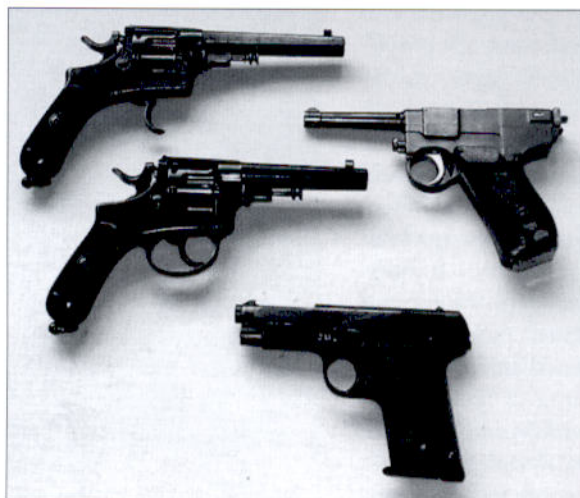
A collection of handguns used by the Arditi: on the top left, a Bodeo mod.1889A for troopers and NCOs with folding trigger, and below this an mod.1889B for officers, with trigger guard: both are 10.35mm calibre. On the upper right is the Glisenti 9mm calibre pistol, while below this is the Beretta mod.1915 9mm calibre gun. (Courtesy MNA Torino, photo Federico Cavallero)
