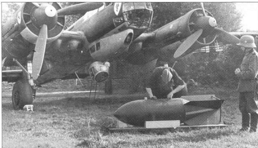
I./KG30 Bombenwart prepares an SC250. The Geschwader's own Platzsicherung (airfield security) detachment was often augmented by army reserve personnel, such as this Landsers with M1916 Stahlhelm . Note the extended dive-brake behind the port engine nacelle, the black and white stripes forming part of the Balkankreuz insignia when closed. (Gregory Pons)
