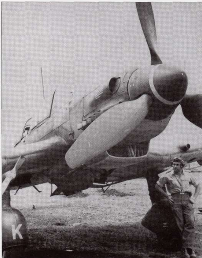
A Feldwebel Flugzeugführer is dwarfed by his Ju87, Russia, 1942. In flight, and even on the ground, it is often difficult to comprehend the scale of the truly enormous Stuka. Its SC250 cargo is here fitted with the rarely seen 'Dinort-Spargel' (asparagus) detonator arm, designed by StG2-Kommodore, Major Oskar Dinort. This improvised device exploded the bomb just above ground level with devastating effect in anti-personnel and vehicle attacks. The 1,000ft average release point ensured minimum safe recovery and reduced target evasion time.
