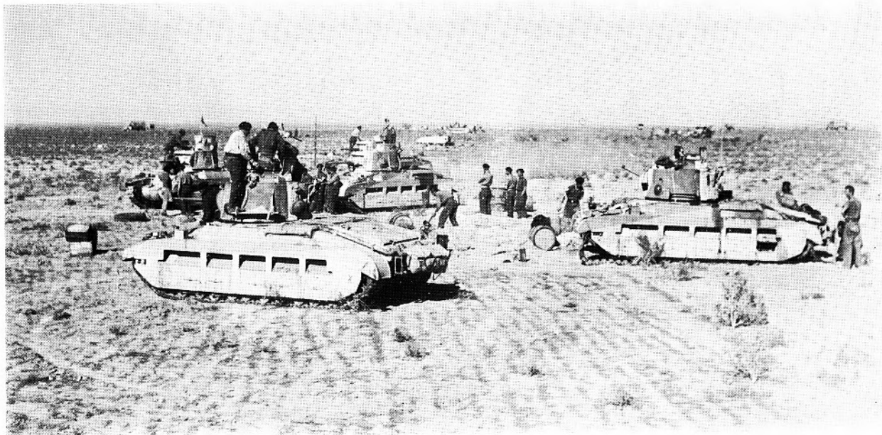
7 RTR refuel, replenish ammunition and repair minor damage at a 'Forward Rally' during the Sidi Barrani operations of December 1940; the broken track (right) is mine damage.
