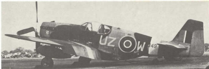
6. A Mustang III, FZ149 of No. 306 (Polish) Sqn. The aircraft has a Malcolm canopy and is plugged into its starter trolley ready to go at a moment's notice. The squadron was used for anti Diver (flying bomb) patrols over southern England in 1944. (IWM)
