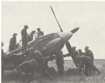
14. RAF Servicing Commandoes swarm round one of the first Spitfire Mk IXs to land in France after D-Day. The aircraft is being refuelled by hand; the cans under the wing are handed to the crew on the fuselage who are using a giant-sized funnel to direct the liquid into the right place. (IWM)
