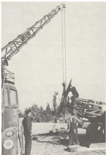
17. A Coles Crane of a Canadian unit (note maple leaf roundel on mudguard) helps the removal of the propeller of a Spitfire Mk IX on a French landing strip. (IWM)
