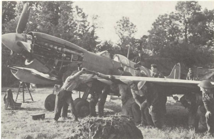
22. An RAF salvage team recovering a damaged Spitfire Mk IX of No. 403 (Canadian) Sqn in France shortly after D-Day. The pilot's seat has been removed, both cannon fairings are missing and the laminated wood propeller blades have severed in what was probably a belly landing. Note lower nose fairing hinged downwards and the jack supporting the centre-section. (IWM)
