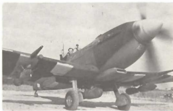
21. Wg Cdr A. G. Page starts a sortie in his Spitfire Mk IXe laden with two 250lb bombs on the wing racks and a 500lb missile on the centreline. The aircraft, which has wheel hub covers in place, shows the pilot's initials painted under the spinner and a rank pennant below the windscreen. (IWM)
