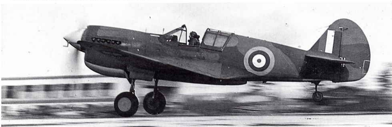
Above Mk. Ia in standard green/brown uppers, pale blue unders. Note red/white/blue roundels on wings. Photo probably taken after Oct. 1942 when sqdn. codes were discontinued for security reasons.
