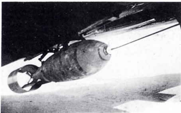
Bomb rack details, 250 lb with extended fuse.
