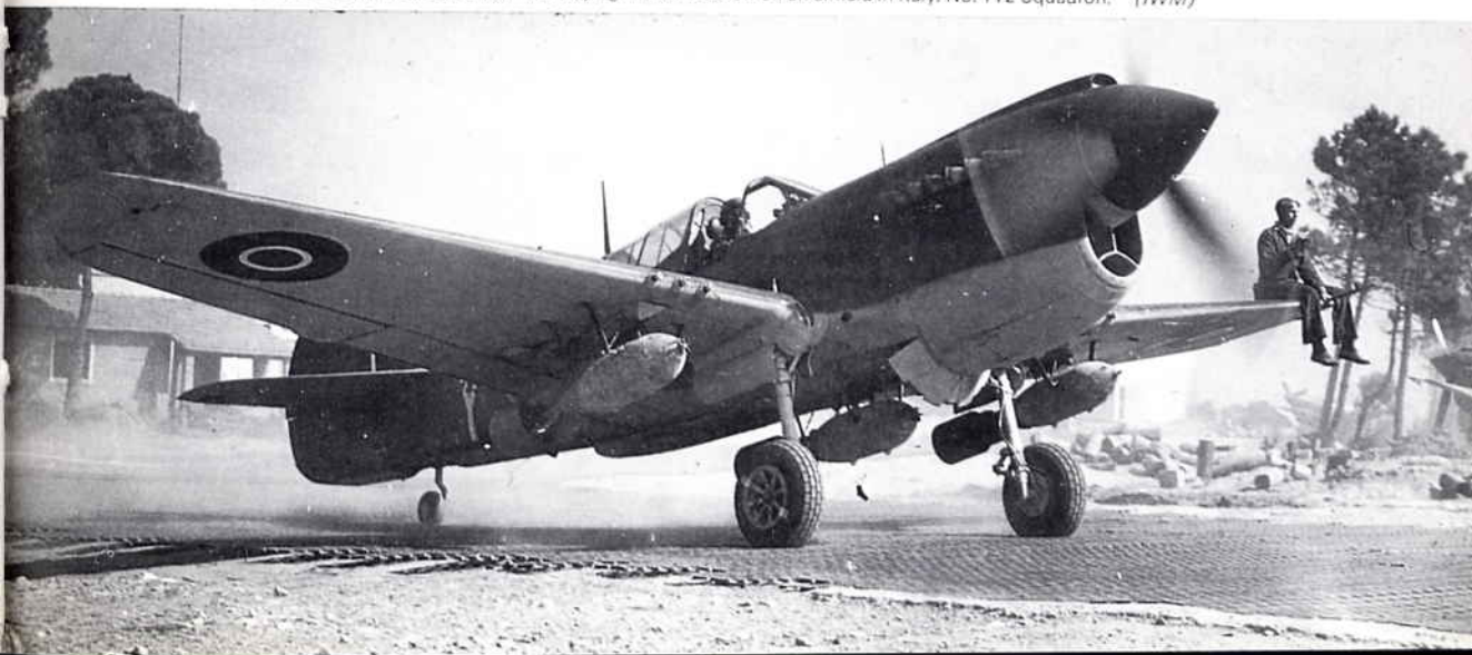
Below Mk. IV bombed up with 3 x 250 lb bombs taxiing out for take-off on an airfield in Italy. No. 112 Squadron. (IWM)
