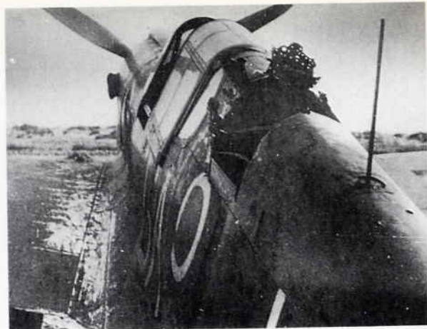
Damaged radio compartment of FR474, GA-Jinx after combat with Fe.190's over Rieti LG, Italy, 7th April 1944. Flown by Fit.Lt. Matthias, No. 112 Squadron.
