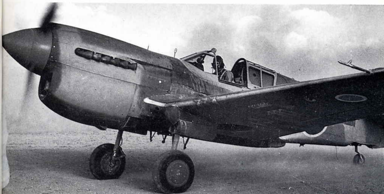
Below Nose detail of a Mk. III, note full span yellow leading edge stripe, wing racks and Azure blue under surfaces. (IWM)
