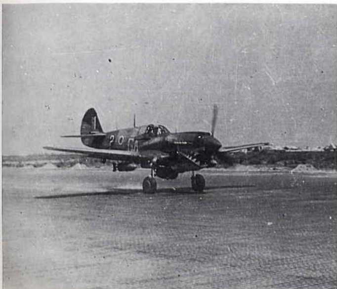
Below Mk. IV, GA-? FX740 taking off from Cutella, Italy. Note bomb load, 1 x 500 lb under fuselage, 2 x 250 lb under wings. Flt.Lt. Ross
