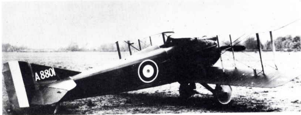
Above & below: These two photographs of A8801 illustrate more clearly the large opaque windshield fitted to the earliest Spads VII built by Blériot & Spad at Addlestone. (Photos: Imperial War Museum Q55997 and Q56000).
