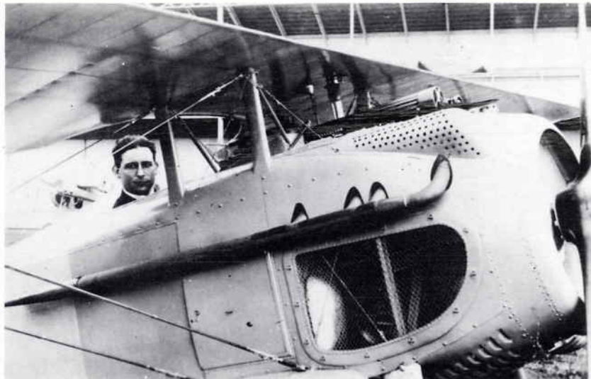
Left: Nose detail of Spad VII with cowling panel removed.
