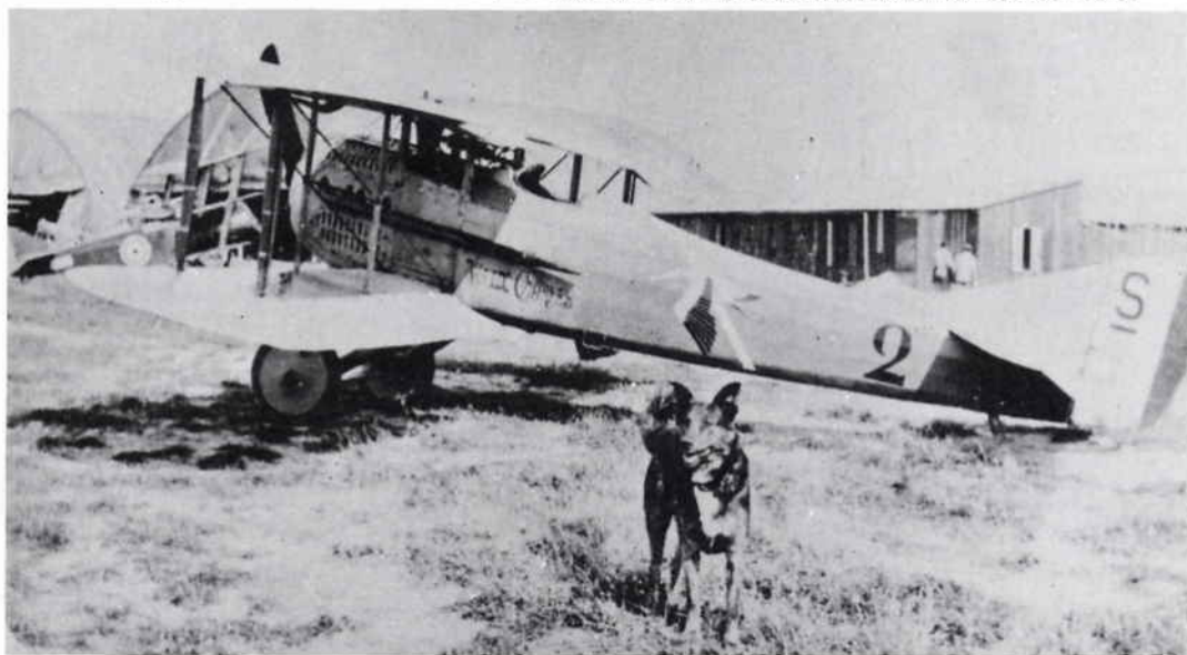
Above: Guynemer's Spad XIII, an early-production aircraft with round wing tips and the original arrangement of centre-section struts. It is believed that this photograph was taken at St. Pol. In the background, at left, is a Sopwith triplane.
