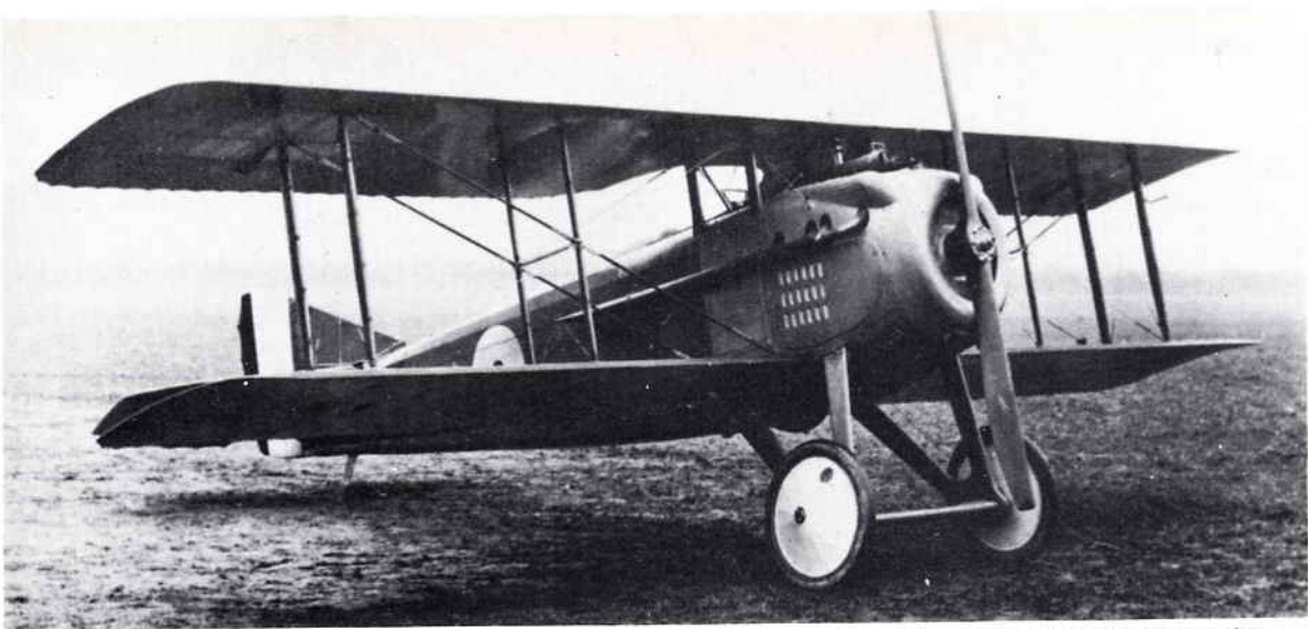
Above: Mann, Egerton Spad VII, probably N6210. This aircraft had a modified radiator cowling with re-entrant leading edge that must have reduced the efficiency of the radiator. (Photo: Imperial War Museum Q.67971).
