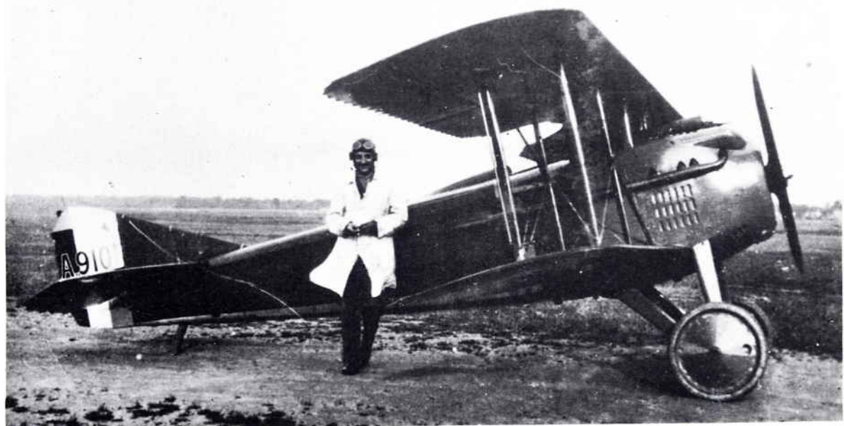
Above: Renumbered A9100, the first Mann, Egerton Spad VII is here seen with its Lewis gun in position. (Photo: Royal Aeronautical Society).
