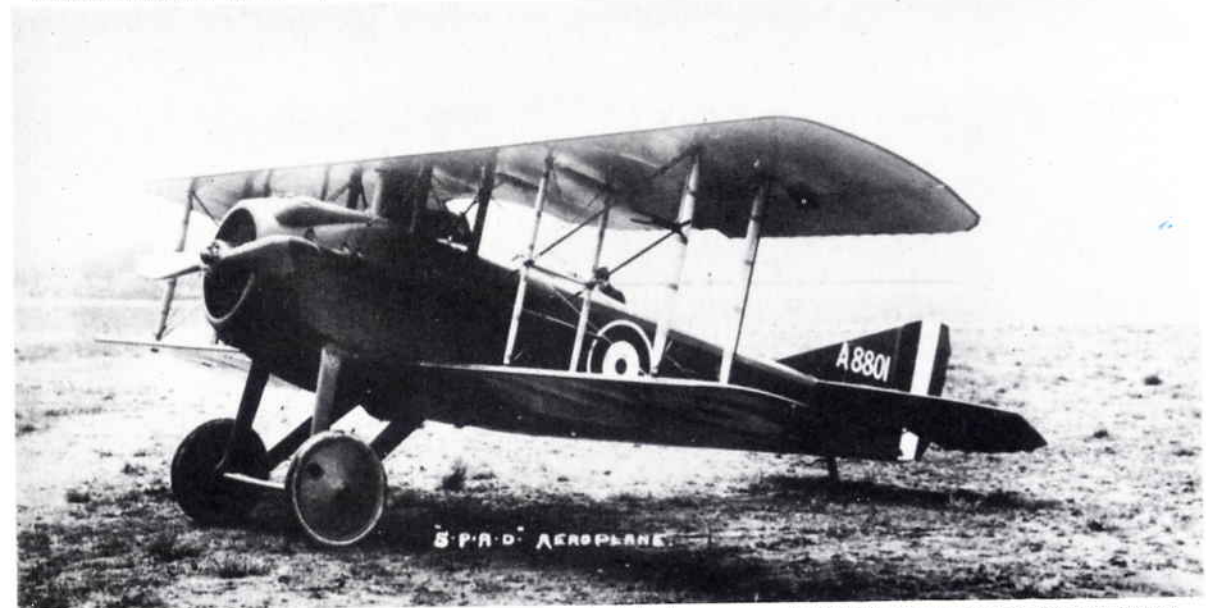
Above & below: These two photographs of A8801 illustrate more clearly the large opaque windshield fitted to the earliest Spads VII built by Blériot & Spad at Addlestone. (Photos: Imperial War Museum Q55997 and Q56000).
