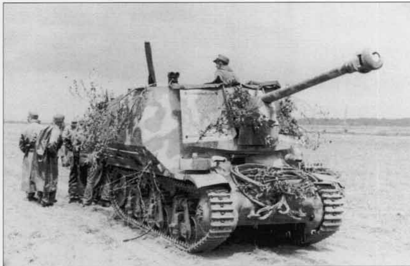
A Marder I, a 75mm Pak 40 (L/46) gun mounted on a captured French Hotchkiss H35 chassis, from 21st Panzer Division to the east of Caen. The division had 24 of these converted self-propelled guns. (Bundesarchiv 1011/493/3365/20)
