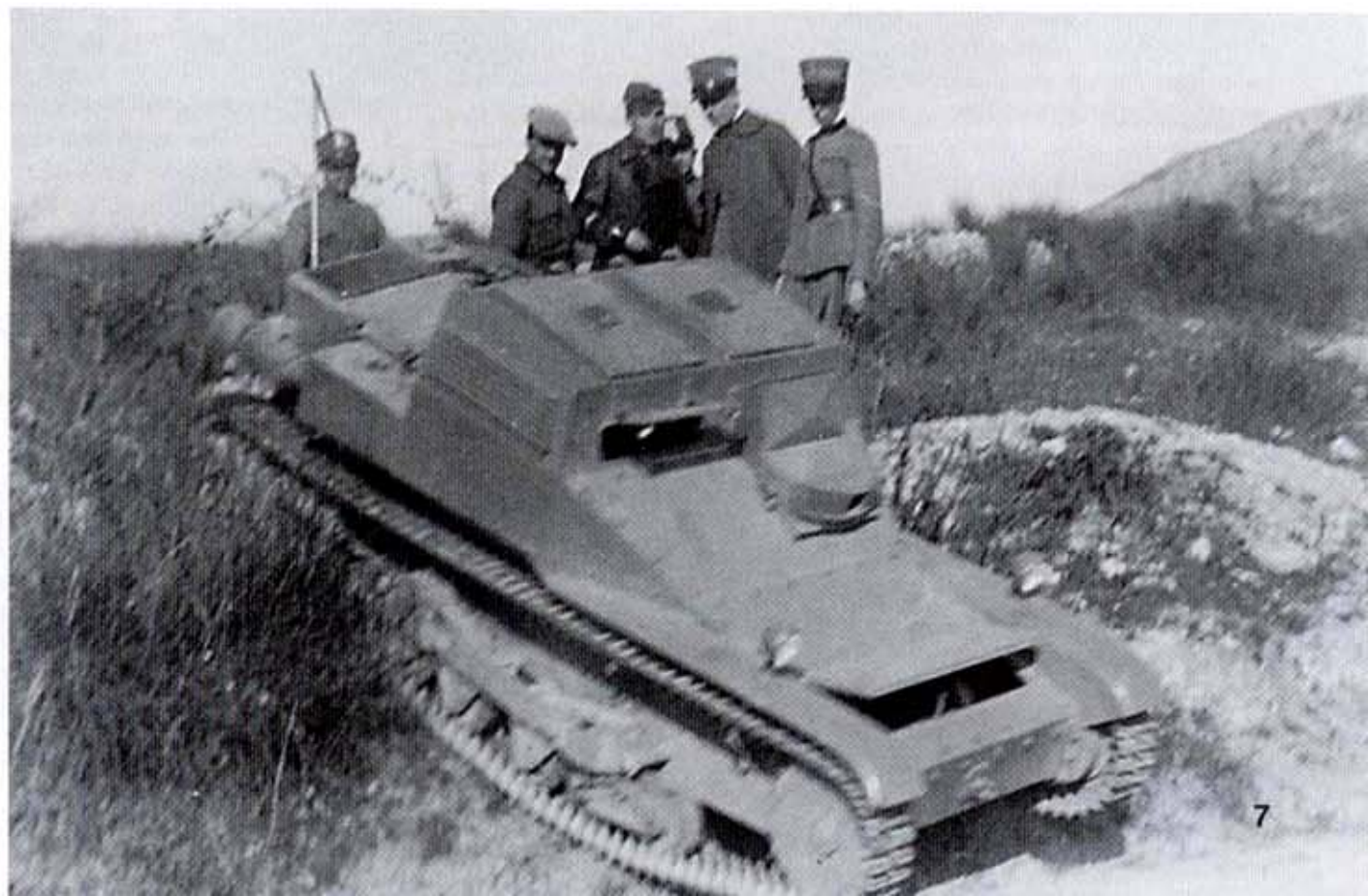
A Carro Veloce 33 pilot vehicle rolls down a rocky hill during its 1933 acceptance trials. This tank fell more properly within the tankette classification, with a weight of 3.4 MT (3.8 tons). Early CV 33s (later designated L 3-33s) were armed with one 6.5MM Fiat-Revelli Model 14 air-cooled aircraft machine gun.
