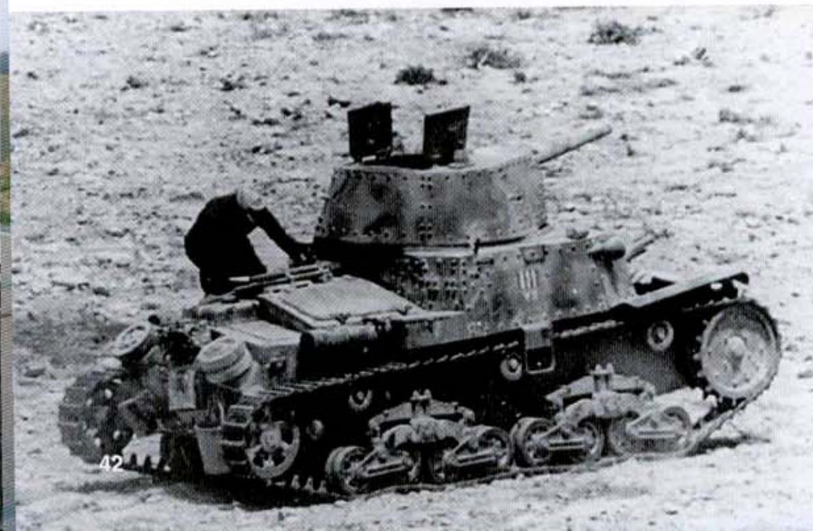
A crewman examines the engine deck of a 3rd production series M 13-40 in North Africa in either 1941 or 1942. A 3rd Platoon insignia is painted on the hull side above the Roman battalion numeral VII (7). The M 13-40 received gray-green mottling over its Saharian Khaki finish. A white cross painted on the turret roof was an aircraft recognition marking. (Bundesarchiv)
