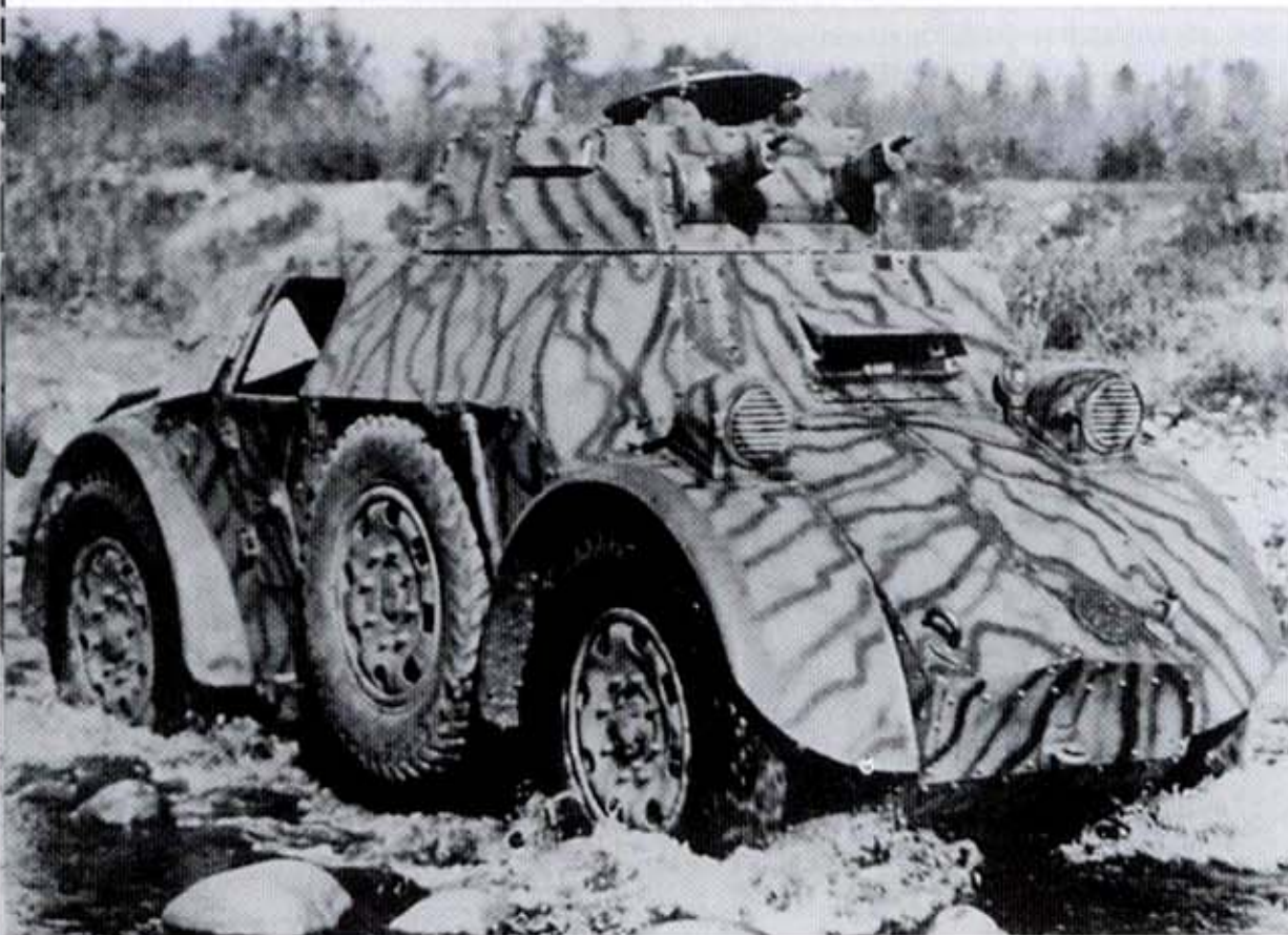
In 1939, Fiat proposed a new armored car to the Regio Esercito , which was based on a specification the War Ministry issued in 1937. This proposal resulted in the Autoblindo (Armored Car) Abm 1 prototype, which is crossing a stream near Turin, Italy – Fiat's home city. The vehicle is painted overall Sahara Sand, with red-brown and gray-green vertical stripes. A spare wheel was mounted on both the left and right hull sides.
