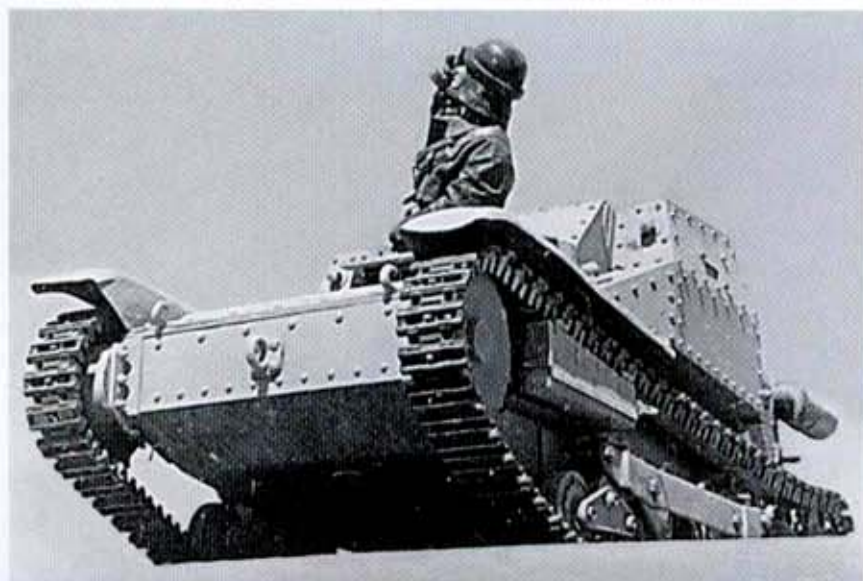
An L 3-35's driver uses a sextant while scanning the North African sky. L 3s generally lacked the roof-mounted anti-aircraft machine gun found on the M tanks; thus, they were vulnerable to strafing attacks. The vehicles' small size was their best defense against air attack. Each L 3 had large drive sprockets mounted at the front. Power from the aft-mounted engine was sent to the gearbox mounted in the front hull. In turn, power was transmitted to the sprockets, which turned the tracks.
