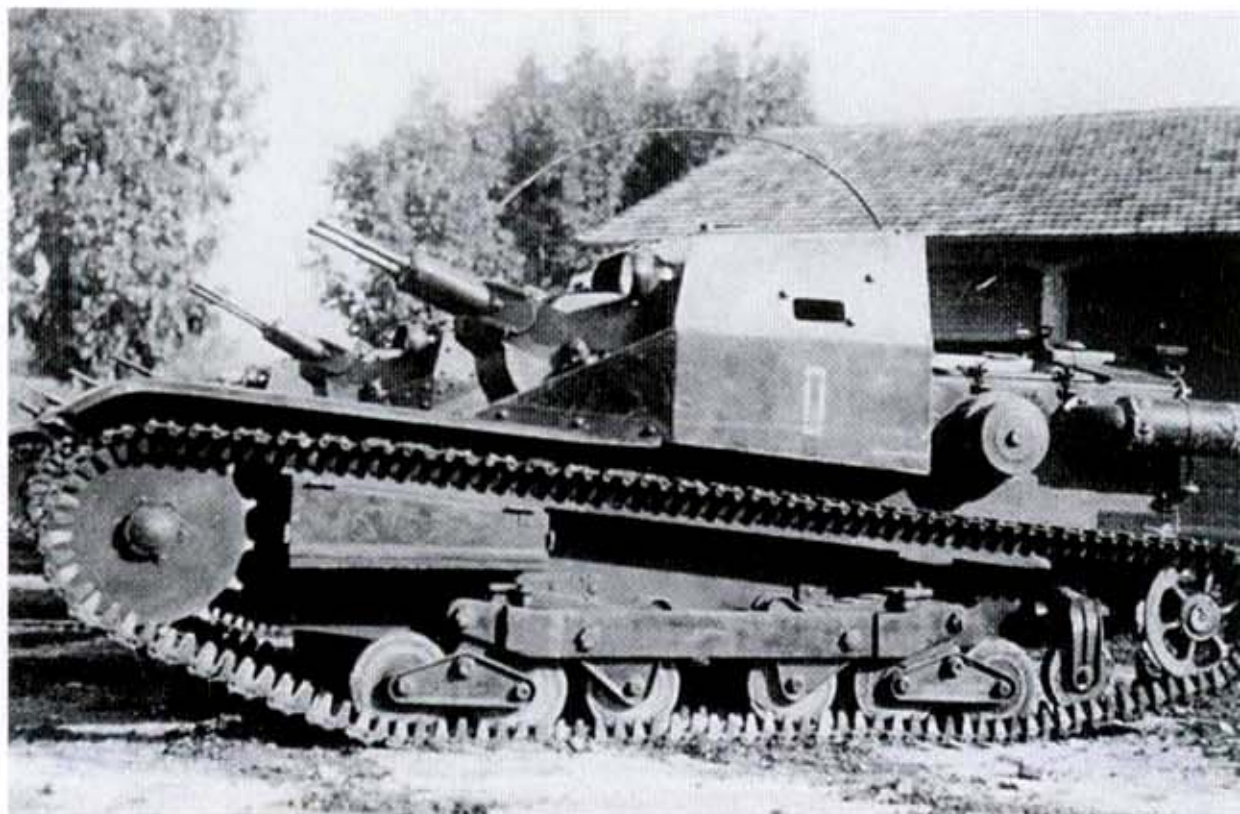
(Above) The second CV 33 production series incorporated minor improvements and changes. These included adding an independent rear track tension idler wheel immediately ahead of the idler wheel. Two 8MM Fiat Model 14/35 machine guns replaced the single 6.5MM Fiat-Revelli Model 14 machine gun. These weapons were The tripod for a heavy machine gun folded and stowed atop the engine deck was a standard fitting for CV 33s.
