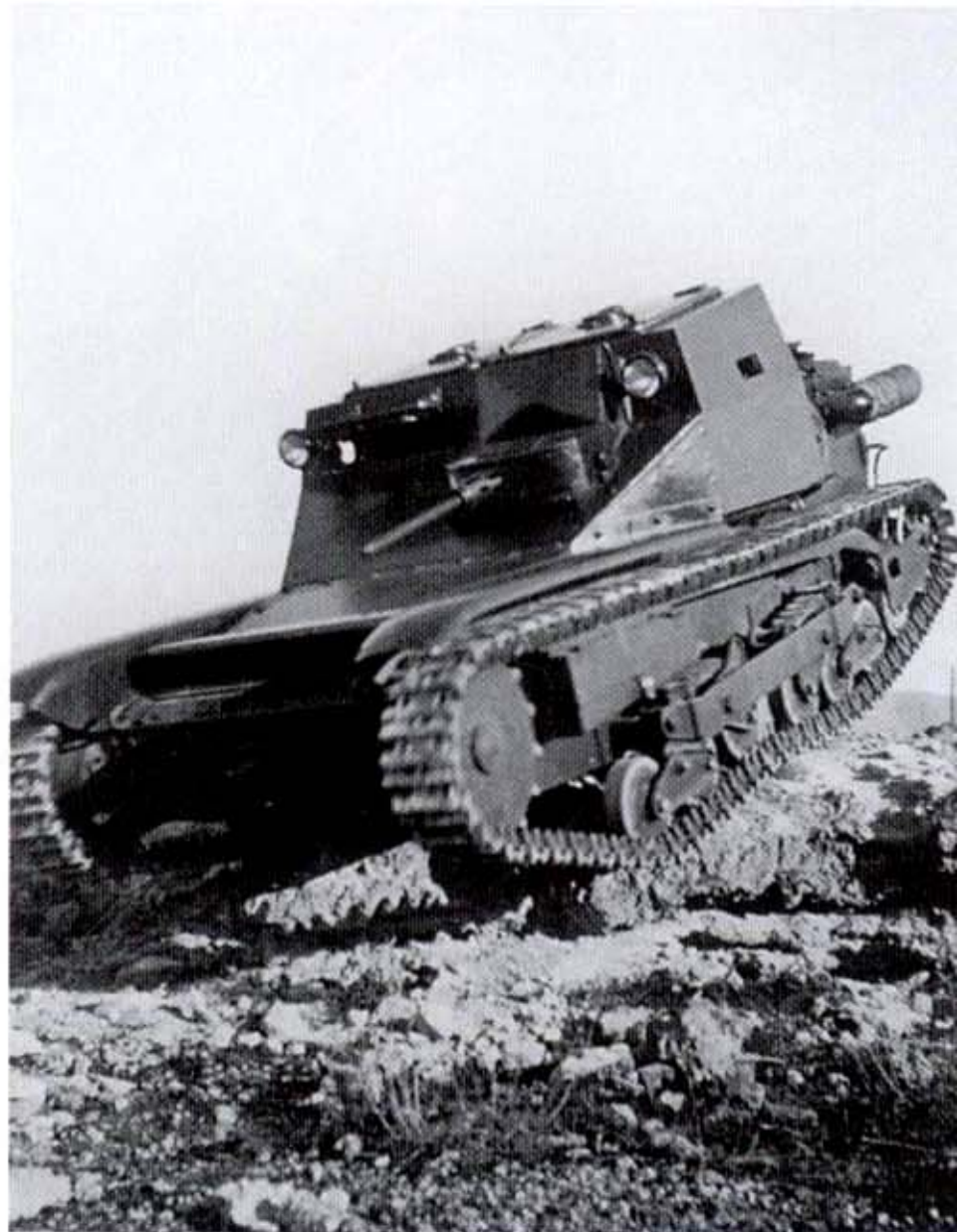
A Carro Veloce 33 pilot vehicle rolls down a rocky hill during its 1933 acceptance trials. This tank fell more properly within the tankette classification, with a weight of 3.4 MT (3.8 tons). Early CV 33s (later designated L 3-33s) were armed with one 6.5MM Fiat-Revelli Model 14 air-cooled aircraft machine gun.
