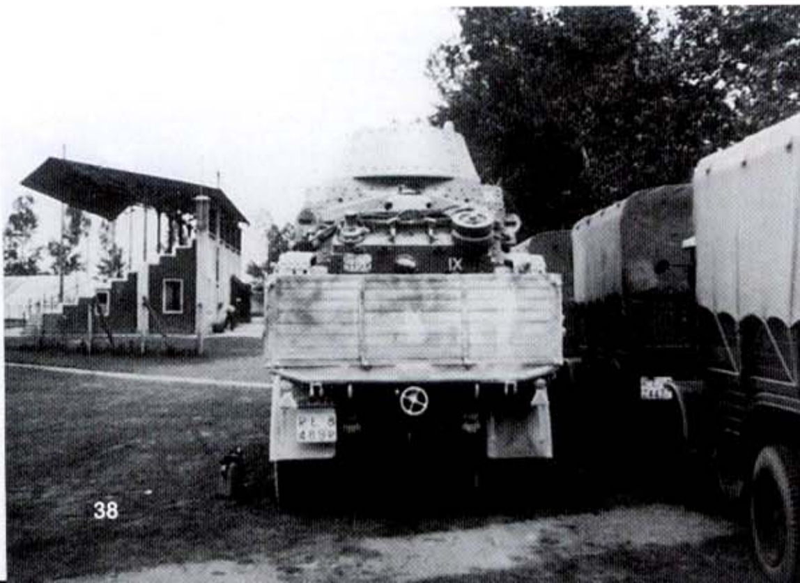
An M 13-40 (R0E TD 3123) assigned to the IX (9th) Battalion, Ariete Armored Division is loaded onto a Viberti tank recovery trailer. A Lancia 3/Ro truck hauled this two axle trailer. The Roman numeral IX that designated the Battalion were painted on both the tank and the trailer. The trailer's white number plate displays the registration R0E TD 8489R. R0E TD (the abbreviation for Regio Esercito ) and R ( Rimorchio ; Trailer) were red, while the numerals were black. A shortage of tank transport trailers required many M 13-40s to advance to front-line positions under their own power. This increased wear and tear on the tanks' tracks and suspensions.
