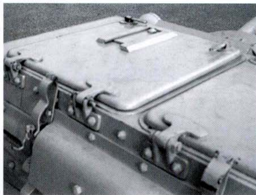
A pair of aft opening hatches were mounted on the L 3-35 fighting compartment roof. An aft-sliding plate in the left hatch roof allowed the commander/gunner to peer upward. The driver's right hatch was identical. This L 3-35 was painted overall Saharian Khaki for service in North Africa.
