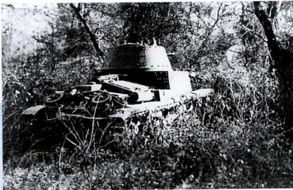
An early production M 13-40 moves through wooded terrain during training. Early production vehicles had long smooth fenders, which were reduced in size on later production tanks. This M 13-40 also has the simple radiator cover on the aft engine deck; later vehicles had the radiator cap moved aft atop this cover and an overhang placed on the cover's right and left edges. Two spare road wheels mounted at the rear of the engine deck facilitated field repairs.
