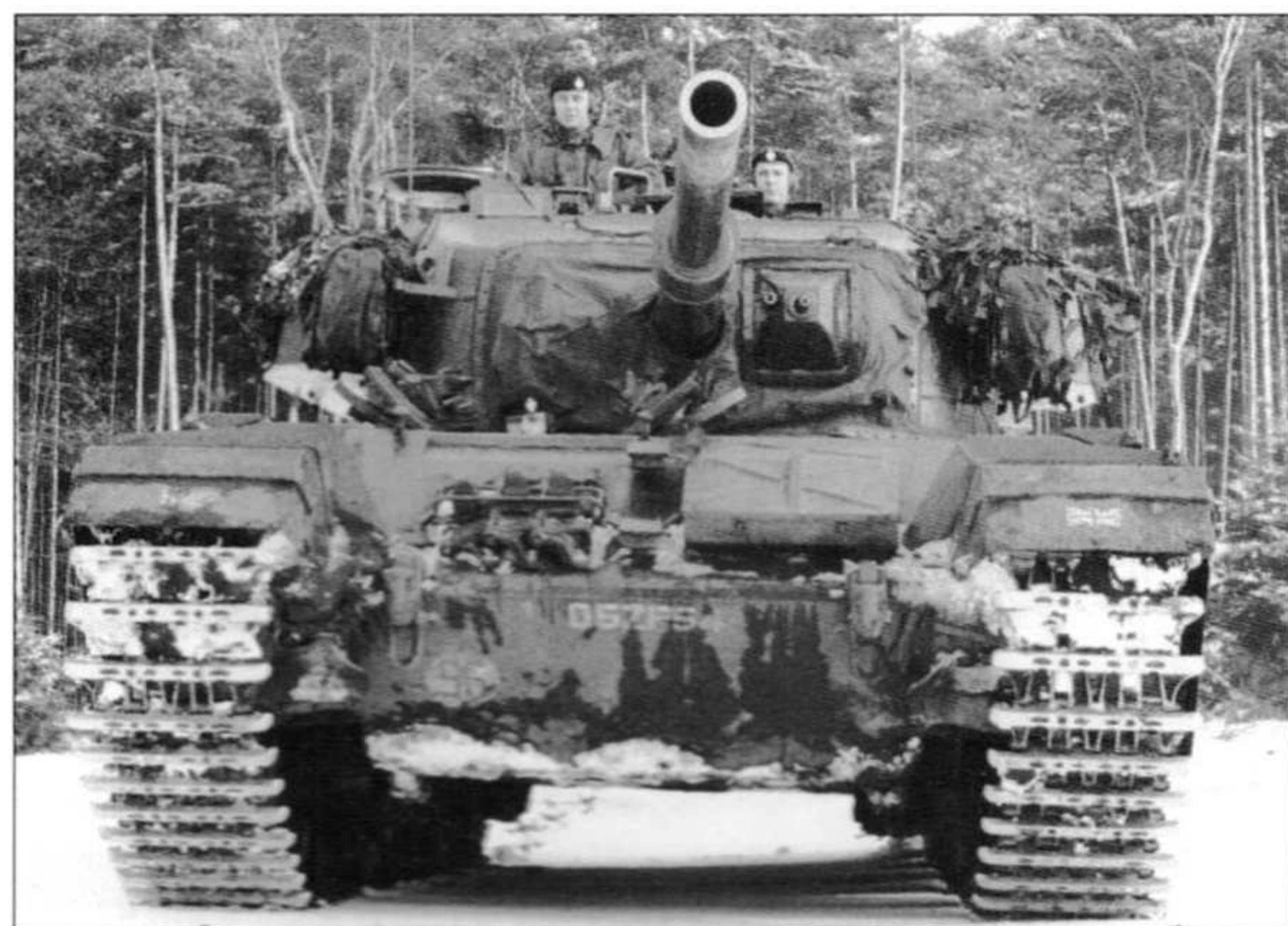
A Centurion Mark 6/2 pauses during an exercise in West Germany during the winter of 1969. The Mark 6/2 incorporated a 0.50-inch ranging gun; visible between the coaxial machine gun and the 105mm main armament.
