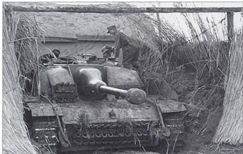
A Sturmgeschütz Ausf.G completed in the autumn of 1943 has the cast gun mantle and an armour deflector in front of the commander's cupola. Concrete has been added on the sloped plate over the driver's position in an attempt to improve protection. (BA)
