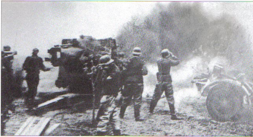
A crew of an 88 mm FlaK 36 in action in Russia. The gun is being fired from its cruciform base with the wheels removed. One set is visible to right of picture. Note the wicker cases in the foreground which contained shells for the gun. (Ian Hogg)
