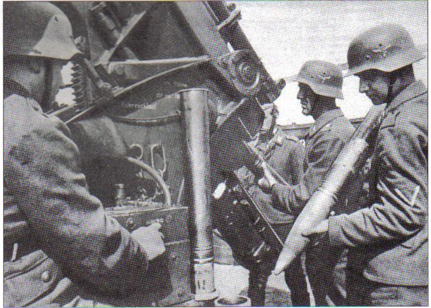
A Luftwaffe crew of a FlaK 37 placing nose cones into the fuse setter. (Ian Hogg)
