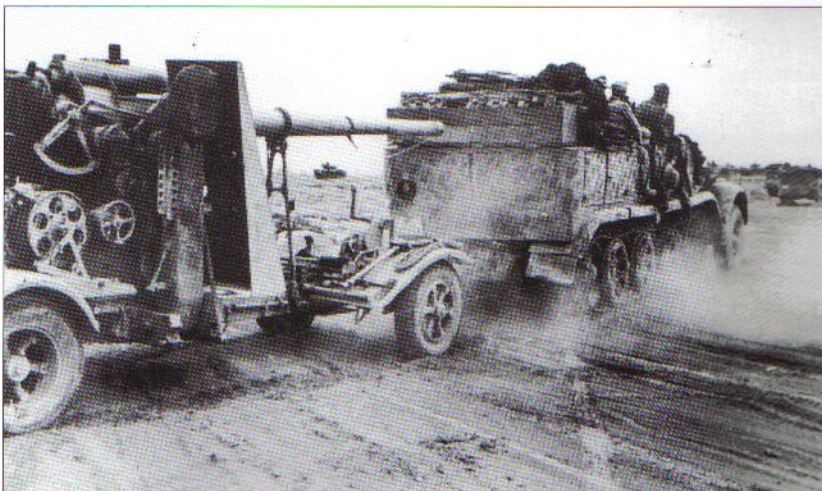
German army on the move in North Africa, January 1942. The 88 is being towed in the standard method, with crew riding on the prime mover stacked with extra fuel, ammunition and personal equipment. Note the 'kill' rings painted on the barrel which indicates the number of targets destroyed by the gun crew.
