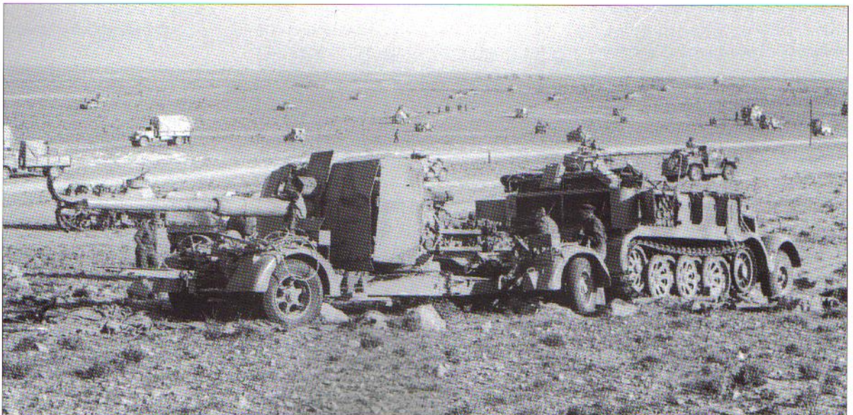
A FlaK 41 captured by the British 8th Army in March 1943 during the advance from El Hamma to Gebes. It has been abandoned along with its prime mover vehicle. Note the folding sides to the gun shield, characteristic of the FlaK 41.
