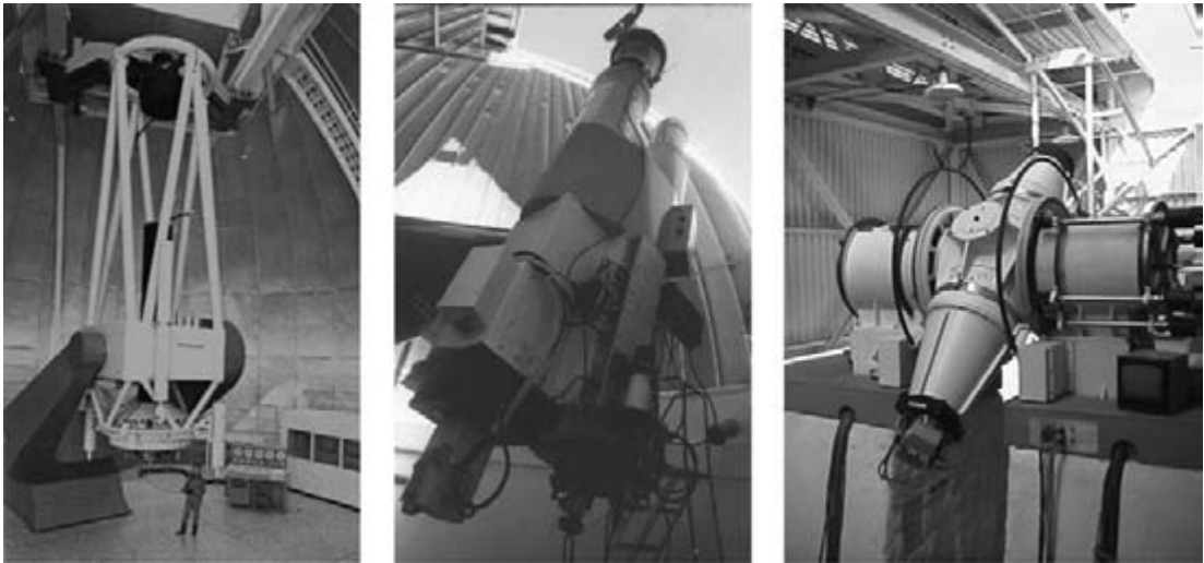
Figure 2.15 Left: the USNO 1.55-m (61-inch) Strand Telescope at Flagstaff, an astrometric reflector used to measure parallaxes since 1964, now equipped with CCDs. Middle: the US Naval Observatory Twin Astrograph at CTIO during the UCAC observations. Right: the 0.2-m (8-inch) Flagstaff Astrometric Scanning Transit Telescope (FASTT), a fully automated telescope, completed in 1981. Photographs courtesy of US Naval Observatory.
