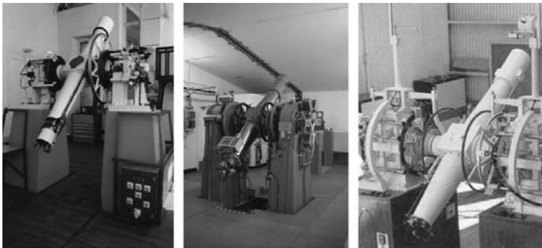
Figure 2.2 Left: the Bordeaux meridian circle was automated in 1978–79, and equipped with the first CCD detectors in 1994. Middle: the Carlsberg Meridian Telescope (formerly the Carlsberg Automatic Meridian Circle), La Palma, started observing in 1984, was upgraded to remote operation in 1997, and further upgraded with a CCD camera operating in drift-scan mode later the same year. Right: the USNO 6-inch transit circle, built in 1898 by Warner & Swasey, used continuously from then until 1995, but no longer actively used for astrometric observations. Photographs courtesy of the respective observatories (Bordeaux, La Palma, US Naval).
