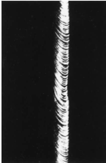
FIGURE 8.9 Slip in a zinc single crystal. (From C. F. Elam, The Distortion of Metal Crystals , Oxford University Press, London, 1935.)
