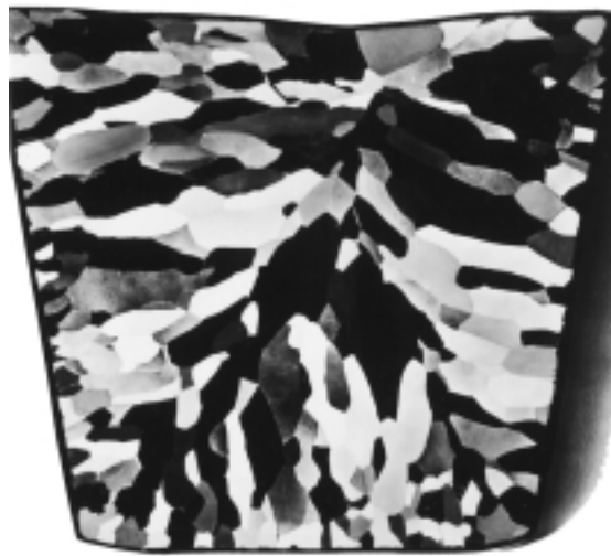
FIGURE 5.14 High-purity polycrystalline lead ingot in which the individual grains may be discerned. 0.7\times . (Reproduced with permission from Metals Handbook , Vol. 9, 9th edition, Metallography and Microstructures , American Society for Metals, Metals Park, OH, 1985.)
