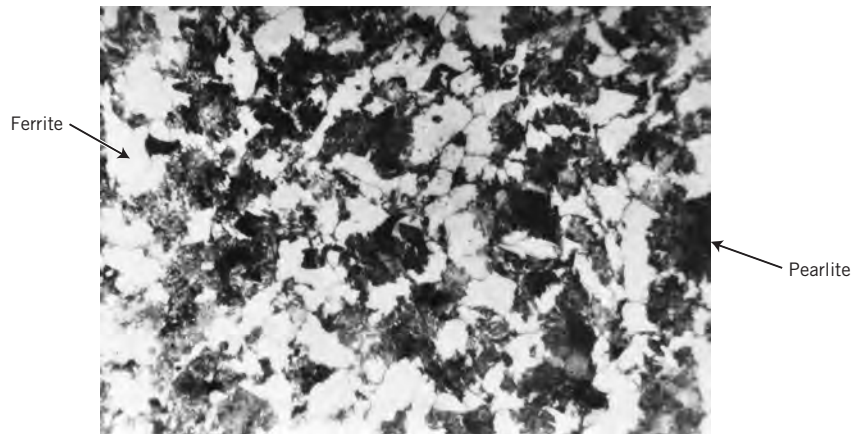
Figure 22.17 Optical photomicrograph of the failed axle central core region, which is composed of ferrite and pearlite (and possibly bainite). 500 \times . [Reproduced with permission from Handbook of Case Studies in Failure Analysis, Vol. 1 (1992), ASM International, Materials Park, OH, 44073-0002.]
