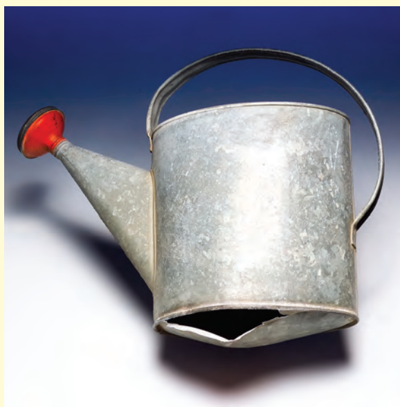
A watering can that ruptured along a side panel-bottom panel seam. Water that was left in the can during a cold late-autumn night expanded as it froze and caused the rupture. (Photography by S. Tanner.)
