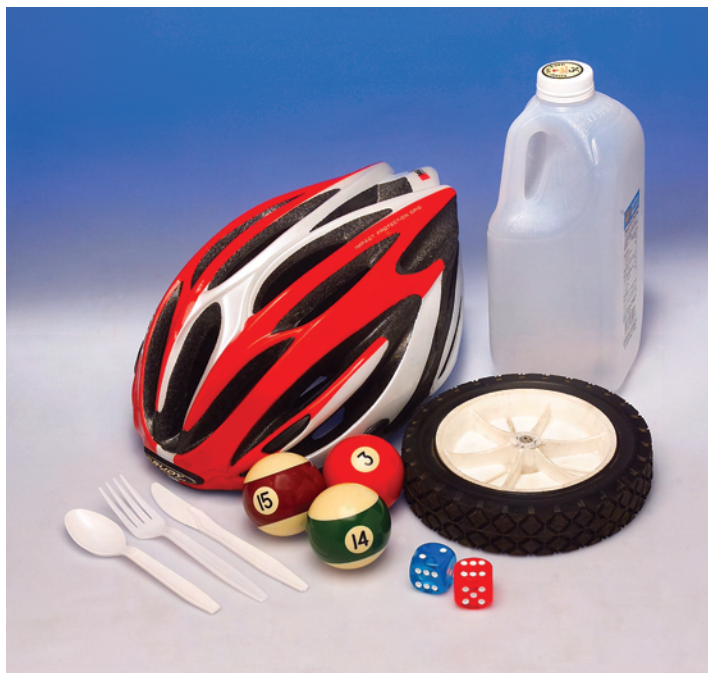
Figure 1.10 Several common objects that are made of polymeric materials: plastic tableware (spoon, fork, and knife), billiard balls, a bicycle helmet, two dice, a lawnmower wheel (plastic hub and rubber tire), and a plastic milk carton. (Photography by S. Tanner.)
