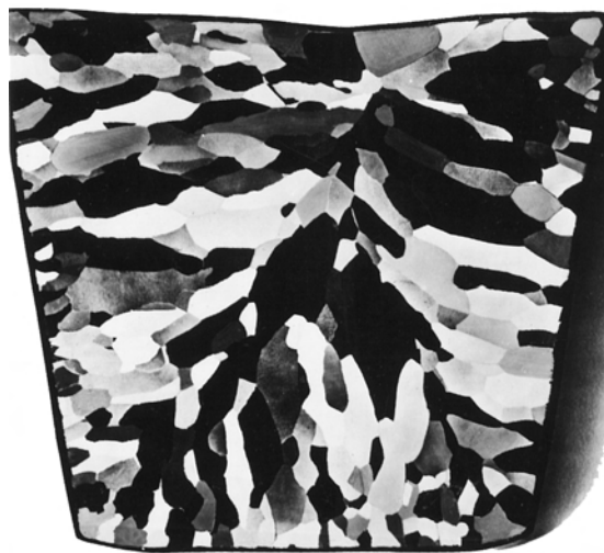
Figure 4.12 High-purity polycrystalline lead ingot in which the individual grains may be discerned. 0.7×. (Reproduced with permission from Metals Handbook , Vol. 9, 9th edition, Metallography and Microstructures , American Society for Metals, Metals Park, OH, 1985.)
