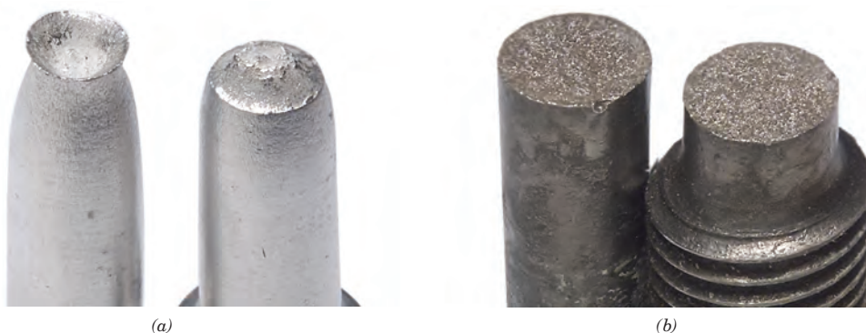
Figure 8.3 (a) Cup-and-cone fracture in aluminum. (b) Brittle fracture in a mild steel.
