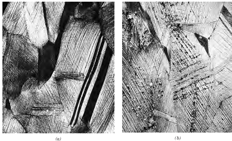
Figure 7.21 Photomicrographs showing several stages of the recrystallization and grain growth of brass. (a) Cold-worked (33% CW) grain structure. (b) Initial stage of recrystallization after heating 3 s at 580°C (1075°F); the very small grains are those that have recrystallized. (c) Partial replacement of cold-worked grains by recrystallized ones (4 s at 580°C). (d) Complete recrystallization (8 s at 580°C). (e) Grain growth after 15 min at 580°C. (f) Grain growth after 10 min at 700°C (1290°F). All photomicrographs 75×. (Photomicrographs courtesy of J. E. Burke, General Electric Company.)
