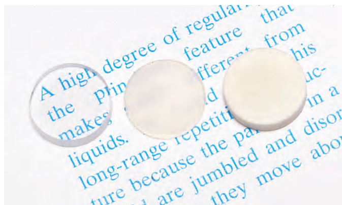
Figure 21.10 Photograph showing the light transmittance of three aluminum oxide specimens. From left to right; single-crystal material (sapphire), which is transparent; a polycrystalline and fully dense (nonporous) material, which is translucent; and a polycrystalline material that contains approximately 5% porosity, which is opaque. (Specimen preparation, P. A. Lessing; photography by S. Tanner.)
