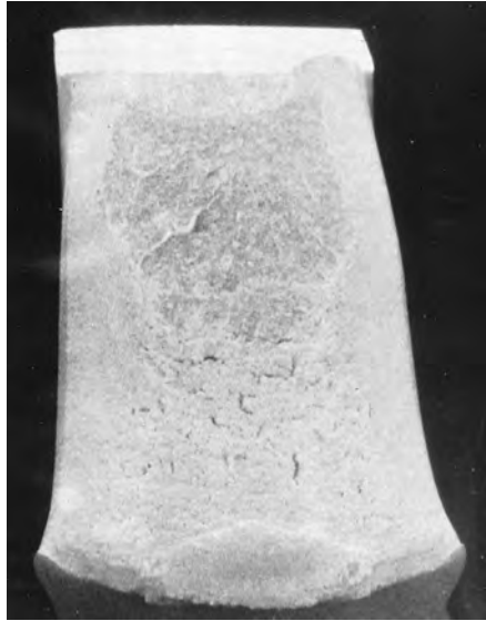
Figure 22.20 Fracture surface of the Charpy impact specimen that was taken from the central core region. [Reproduced with permission from Handbook of Case Studies in Failure Analysis, Vol. 1 (1992), ASM International, Materials Park, OH, 44073-0002.]
