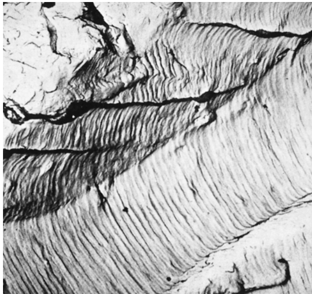
Figure 8.22 Transmission electron fractograph showing fatigue striations in aluminum. Magnification unknown. (From V. J. Colangelo and F. A. Heiser, Analysis of Metallurgical Failures , 2nd edition. Copyright © 1987 by John Wiley & Sons, New York. Reprinted by permission of John Wiley & Sons, Inc.)
