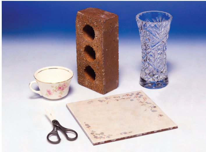
Figure 1.9 Common objects that are made of ceramic materials: scissors, a china tea cup, a building brick, a floor tile, and a glass vase. (Photography by S. Tanner.)
