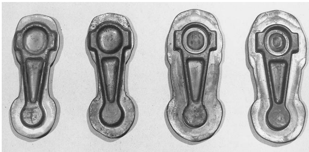
Fig. A.5 Parts that were blocker and finish forged in forging trials
