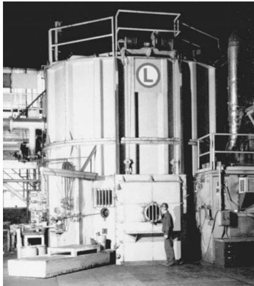
Fig. 20.12 10,000 ton isothermal forging press, designed, constructed, and operated by Ladish. Courtesy of Ladish Co.
