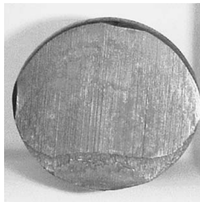
Fig. 13.1 Sheared surface of a billet [Duvari et al., 2003]
