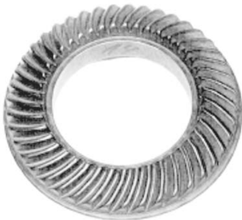
Fig. 23.24 Bevel gear with teeth made on an axial closed-die rolling machine [Husmann, 1999]
