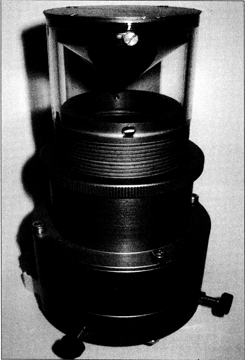
Figure 9. Detailed view of the 360 degree camera system of the Sahabot 2.
