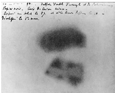
c / Becquerel's photographic plate. In the exposure at the bottom of the image, he has found that he could absorb the radiations, casting the shadow of a Maltese cross that was placed between the plate and the uranium salts.
