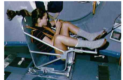
c / Astronaut Tamara Jernigan measures her inertial mass aboard the Space Shuttle.
