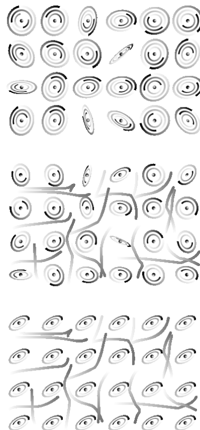
j / The planetary model applied to a nonmetal, 1, an unmagnetized metal, 2, and a magnetized metal, 3. Note that these figures are all simplified in several ways. For one thing, the electrons of an individual atom do not all revolve around the nucleus in the same plane. It is also very unusual for a metal to become so strongly magnetized that 100% of its atoms have their rotations aligned as shown in this figure.
