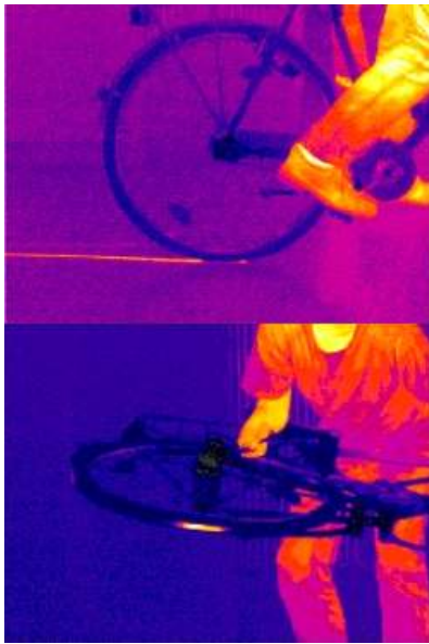
c / As in figure b, an infrared camera distinguishes hot and cold areas. As the bike skids to a stop with its brakes locked, the kinetic energy of the bike and rider is converted into heat in both the floor (top) and the tire (bottom).
