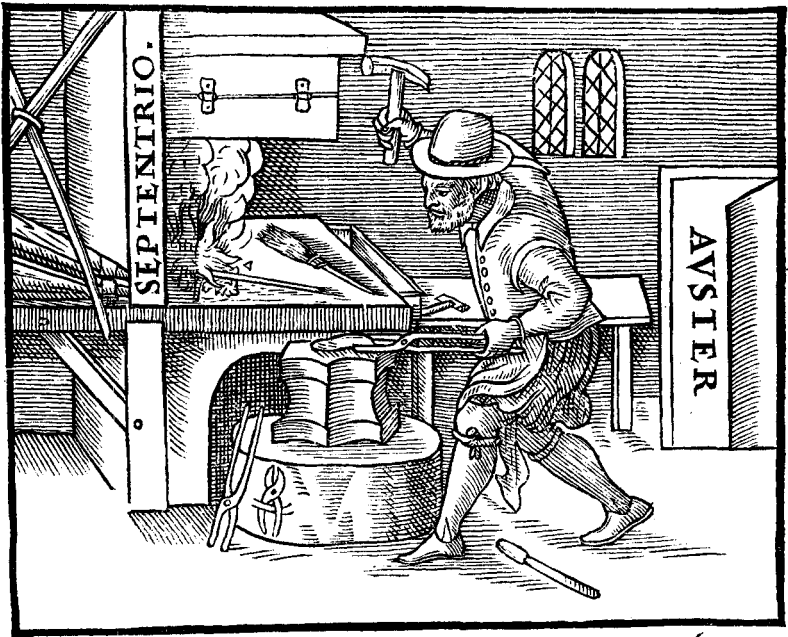
Figure 2-2. An illustration from Gilbert's book, De Magnete , showing how hot iron, when beaten, can be made magnetic. Courtesy Burndy Library, Norwalk, Connecticut.
