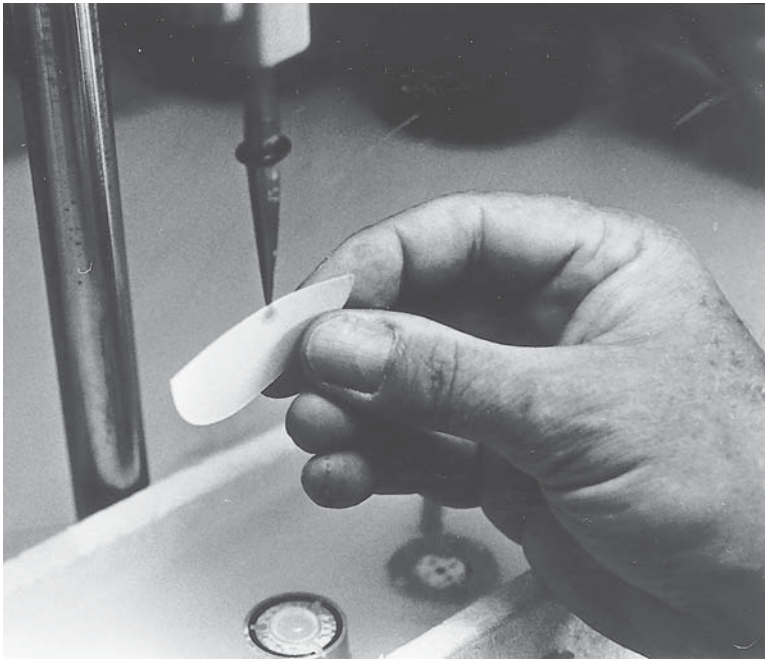
Fig. 4. The direct blotting of a sample on a holey carbon support film with a filter paper, immediately prior to plunge freezing.
