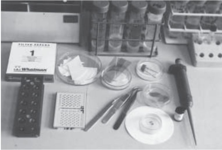
Fig. 1. An example of some of the small equipment needed for the production of negatively stained specimens.
