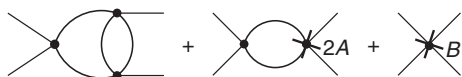
Figure 3 A two-loop graph and its counter-terms. The label B indicates that it is the two-loop overall counter-term for this graph.
