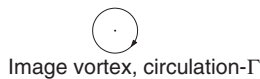
Figure 16 The motion of a point vortex near an infinite straight wall. The vortex moves, at constant speed, maintaining a constant distance from the wall. Other possible trajectories are shown; they are all straight lines parallel to the wall. The motion can be thought of as being induced by an opposite-circulation “image” vortex at the reflected point in the wall.
