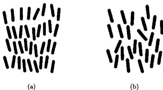
Fig. 9.8. Schematic snapshot of a molecular configuration in a smectic liquid crystal (a) and in a nematic liquid crystal (b).
