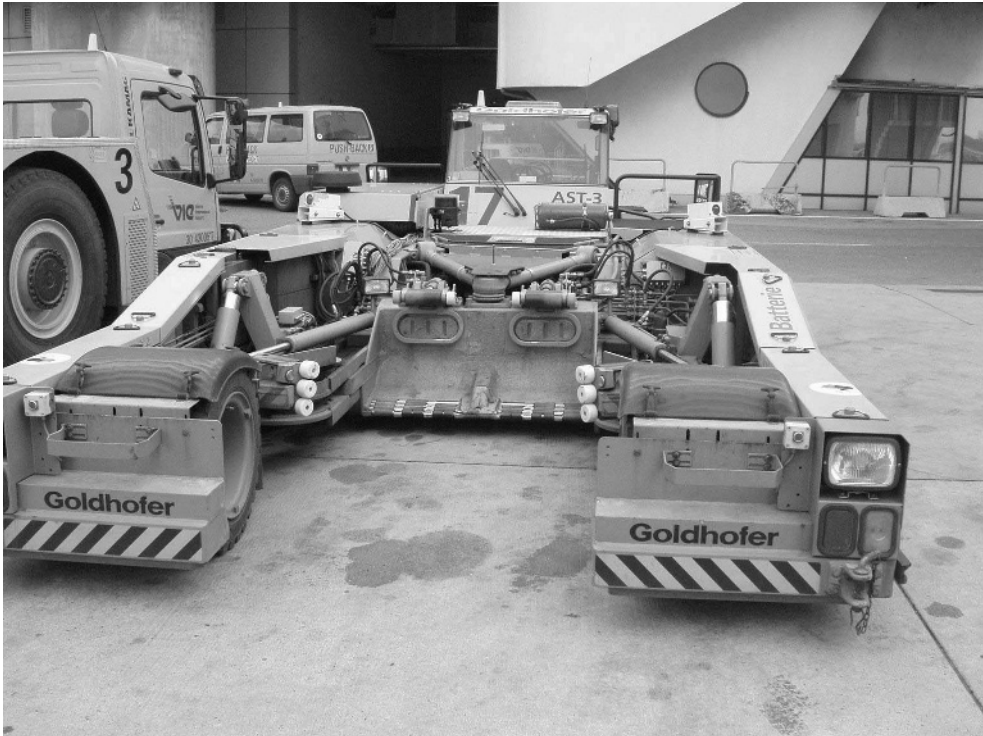
Figure 9-8 Heavy Goldhofer towbarless tractor (Photo: A. Kazda)
