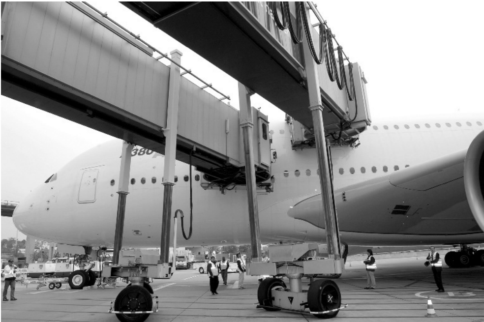
Figure 9-4 The upper deck boarding bridge for Airbus 380 must be able to reach the 8 m (26.2ft) doorsill height (Photo: Courtesy Airbus company)
