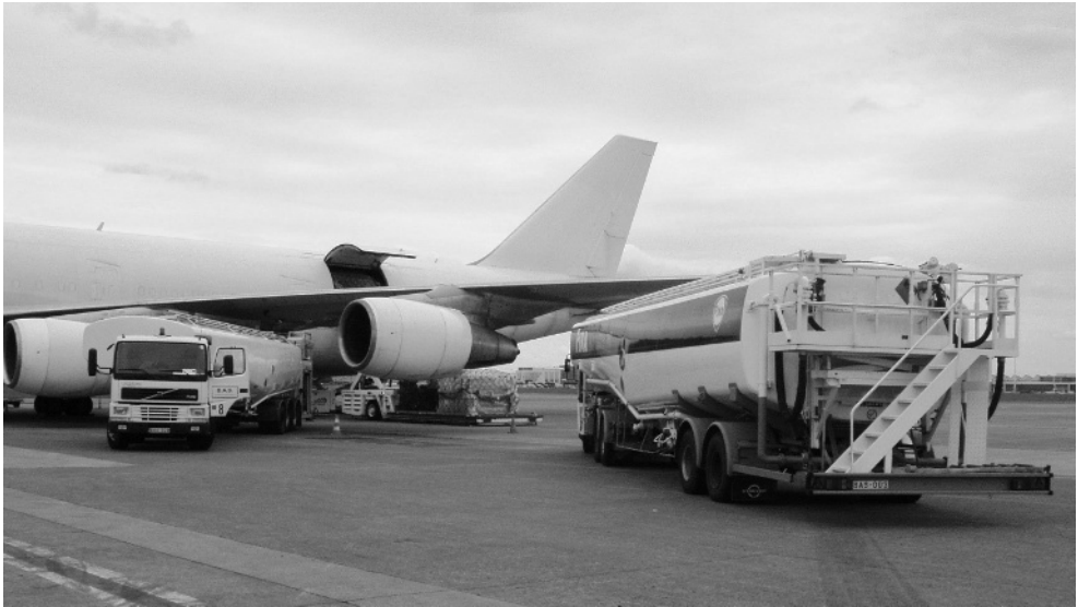
Figure 10-4 B-747 refuelling requires sometimes more than one tanker (Photo: A. Kazda)
