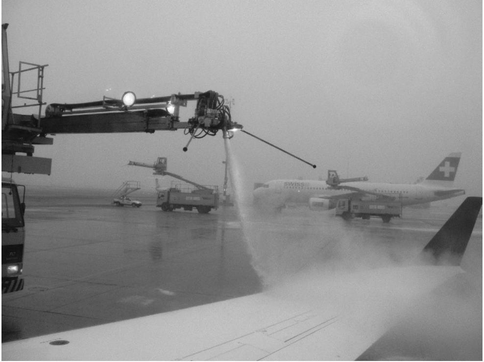
Figure 18-11 Aircraft de-icing at Vienna airport, Type I fluid is used (Photo: A. Kazda)
