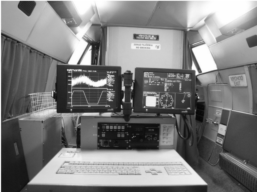
Figure 17-9 Flight inspection aircraft with measuring systems (Photo: J. Šulc)
