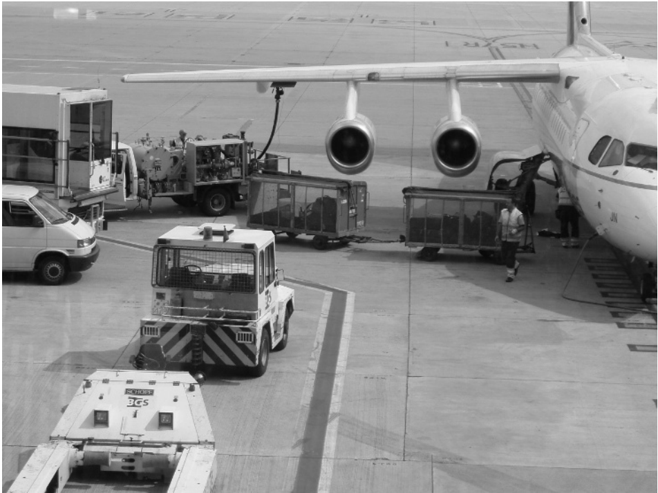
Figure 10-2 Aircraft refuelling by fuel dispenser blocks off a minimum of space during operation (Photo: A. Kazda)
