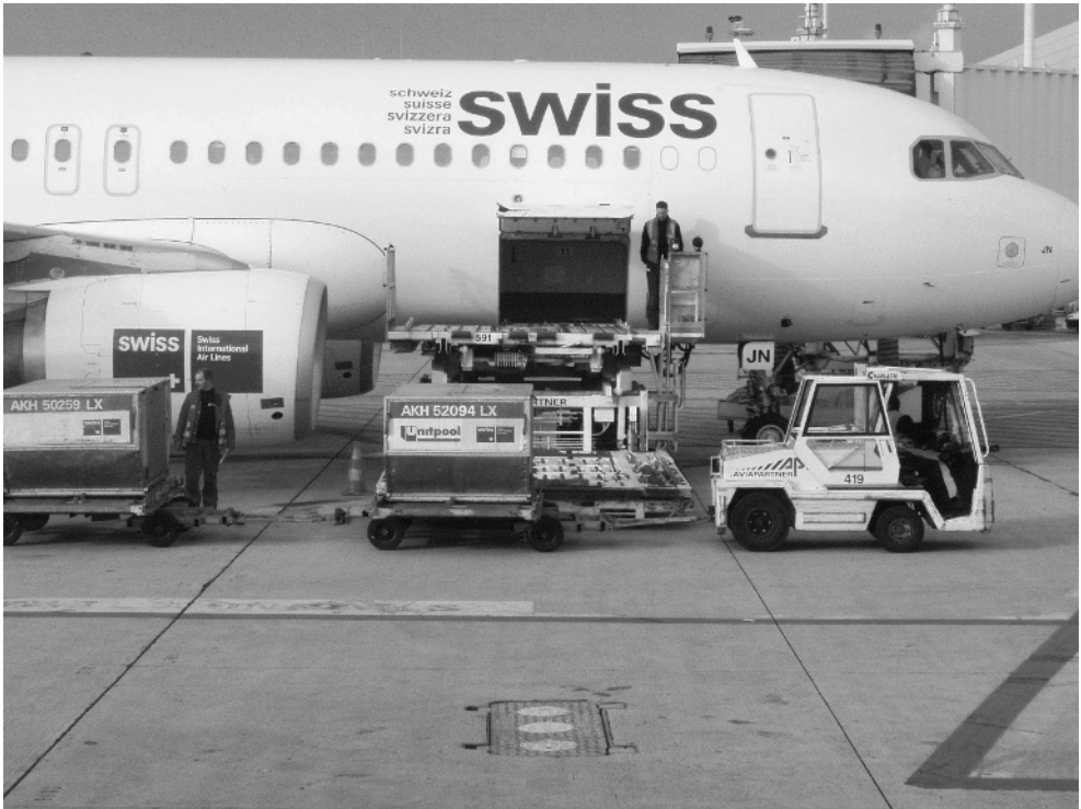
Figure 11-3 Contoured ULDs on roller-bed dollies (Photo: A. Kazda)
