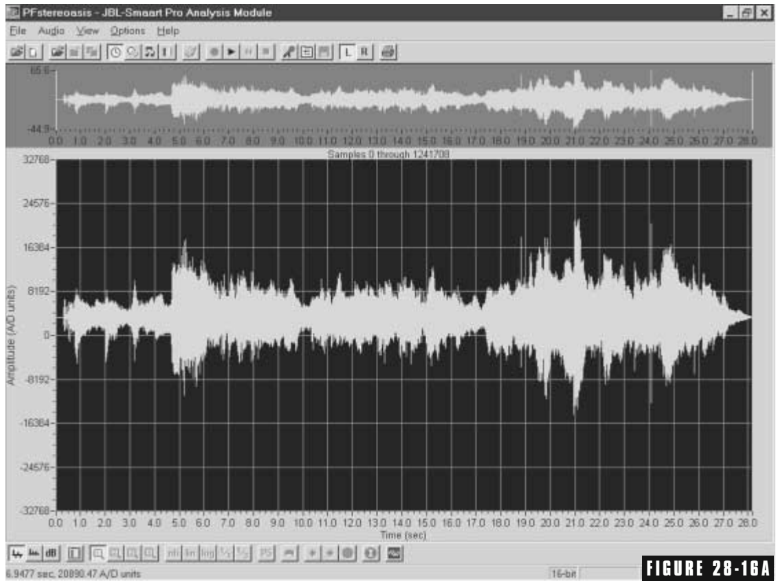
The convolution of the binaural room impulse responses with music generates the left (A) and right (B) wave files which can be played back for auralization.
