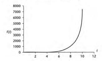
Notice that the term  $\frac{1}{3}e^{-t/2}\Big(\cos\frac{\sqrt{3}}{2}t+\sqrt{3}\sin\frac{\sqrt{3}}{2}t\Big)$  represents damped harmonic motion and is called the **transient** term whereas the term  $\frac{e^t}{3}$  represents a **steady-state** term, so called because as the transient term decays the steady-state term remains the dominant part of the solution. The steady-state solution is a direct consequence of the term on the right-hand side of the differential equation.
