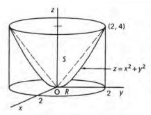
$$S = \int_{R} \int \sqrt{1 + \left(\frac{\partial z}{\partial x}\right)^{2} + \left(\frac{\partial z}{\partial y}\right)^{2}} dx dy$$
