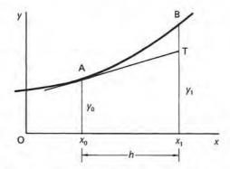
In Euler's method, we use the slope  $(y')_0$  at A  $(x_0, y_0)$  across the whole interval h to obtain an approximate value of  $y_1$  at B. TB is the resulting error in the result.
