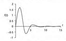
The effect of the 5f'(t) in the differential equation is to introduce **damping** into the oscillatory motion so causing the oscillations to decay. Let's try another example.
