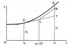
In the Euler–Cauchy method, we use the slope at A  $(x_0, y_0)$  across half the interval and then continue with a line whose slope approximates to the slope of the curve at  $x_1$ .
