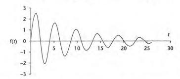
Again, the effect of the f'(t) in the differential equation is to introduce damping into the oscillatory motion so causing it to decay. Also because the coefficient of f'(t) is smaller in this example, the damping is less severe.
