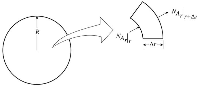
Figure 8.38. Mass transfer from a spherical drop.
