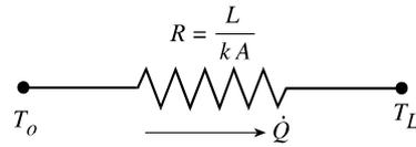
Figure 8.8. Electrical circuit analog of the plane wall.
