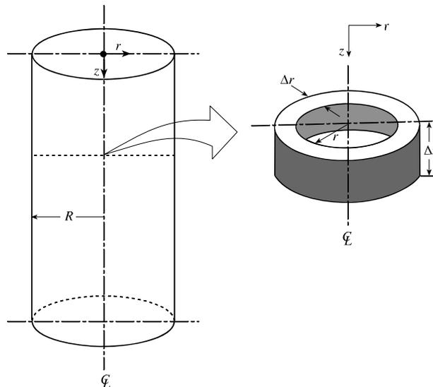
Figure 9.17. Forced convection mass transfer in a pipe.
