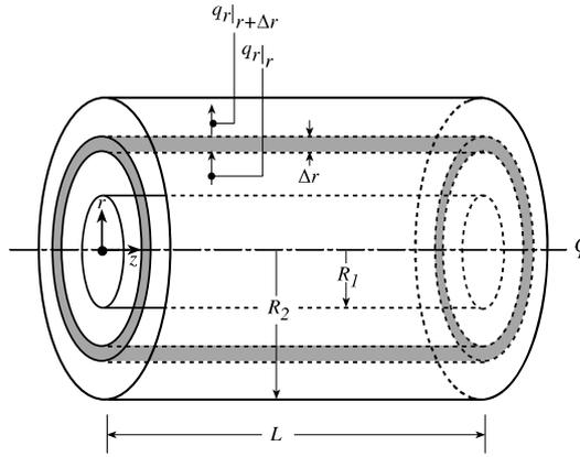
Figure 8.17. Conduction in a hollow cylindrical pipe.
