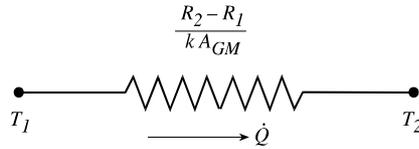
Figure 8.23. Electrical circuit analog of the spherical wall.
