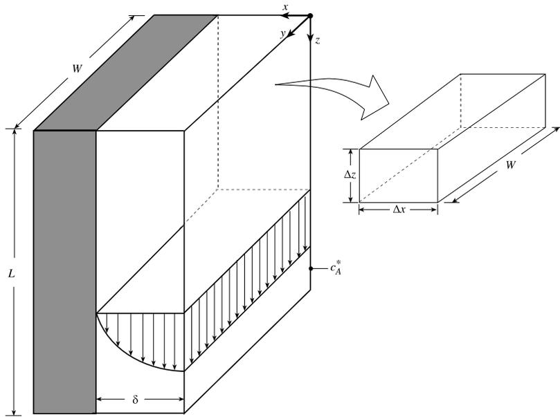
Figure 9.20. Diffusion into a falling liquid film.
