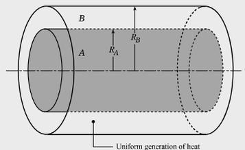
Heat is generated uniformly in region B at a rate  $\mathfrak{R}$  ( $\text{W}/\text{m}^3$ ). Cooling fluid at a temperature of  $T_\infty$  flows over the surface of the cylinder with an average heat transfer coefficient  $\langle h \rangle$ .
