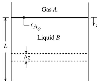
Figure 9.14. Diffusion and reaction in a liquid.
