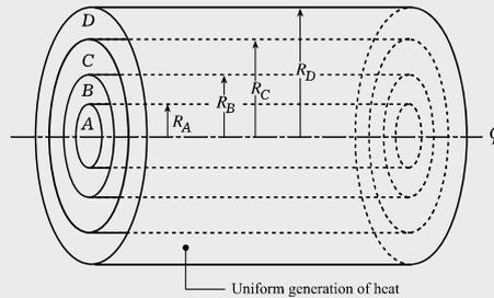
Heat is generated uniformly in region D at a rate  $\mathfrak{R}$  ( $\text{W}/\text{m}^3$ ). Cooling fluid at a temperature of  $T_\infty$  flows over the surface of the cylinder with an average heat transfer coefficient  $\langle h \rangle$ .
