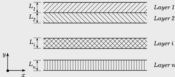
In engineering calculations, it is convenient to treat such a layered structure as a homogeneous material with two different effective thermal conductivities: one describing heat flow within the plane, i.e., in the  $x$ -direction, and the other describing heat flow through the thickness of the plate, i.e., in the  $y$ -direction.
