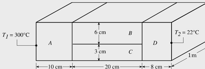
Figure 8.13. Heat conduction through a composite wall.
