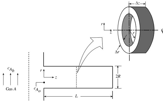
Figure 8.34. Diffusion and reaction in a cylindrical pore.
