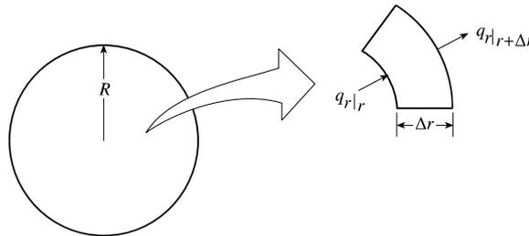
Figure 11.4. Unsteady-state conduction in a sphere with generation.
