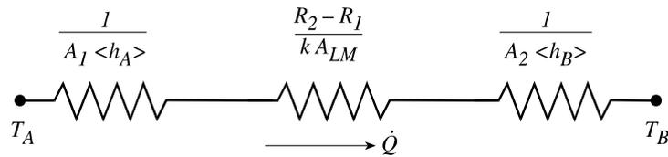
Figure 8.19. Electrical circuit analogy for Eq. (8.2-40).
