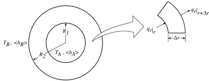
**Figure 8.22.** Conduction through a hollow sphere.
