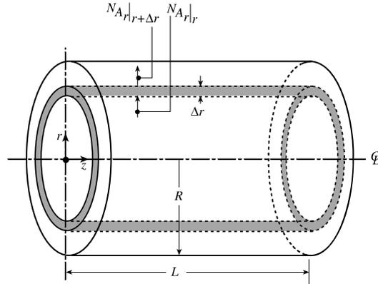
Figure 10.8. Unsteady diffusion into a solid cylinder.
