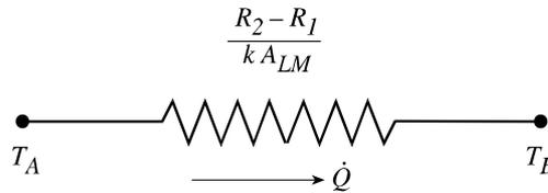
Figure 8.18. Electrical circuit analog of the cylindrical wall.
