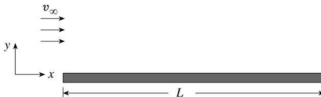
Figure 3.1. Flow on a flat plate.
