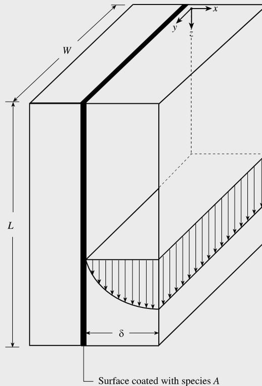
**Figure 2.7.** Solid dissolution into a falling film.
