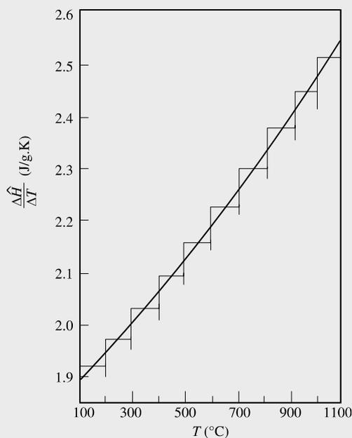
Each line represents the average value of  $d\widehat{H}/dT$  over the specified temperature range. The smooth curve should be drawn so as to equalize the area under the group of bars. From the figure, the heat capacity at constant pressure at 500°C is 2.15 J/g·K.
