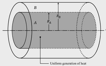
Heat is generated uniformly in region A at a rate  $\mathfrak{R}$  ( $\text{W}/\text{m}^3$ ). Cooling fluid at a temperature of  $T_\infty$  flows over the surface of the cylinder with an average heat transfer coefficient  $\langle h \rangle$ .
