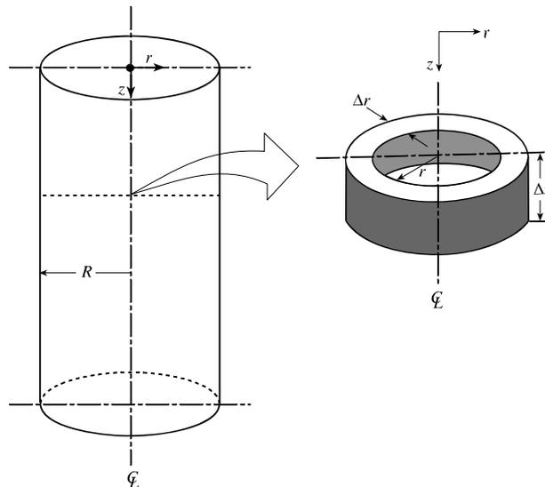
Figure 9.9. Forced convection heat transfer in a pipe.
