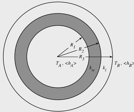
Figure 8.20. Conduction through an insulated cylindrical pipe.
