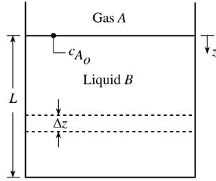
Figure 11.5. Unsteady diffusion with a homogeneous reaction.
