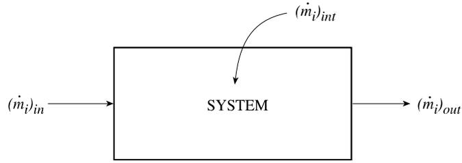
Figure 6.1. Steady-state flow system with fixed boundaries.
