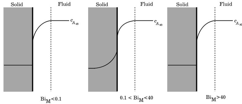
Figure 10.6. Effect of  $Bi_M$  on the concentration distribution.
