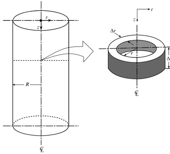
Figure 11.1. Unsteady-state flow in a circular pipe.
