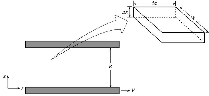
Figure 10.1. Unsteady Couette flow between parallel plates.
