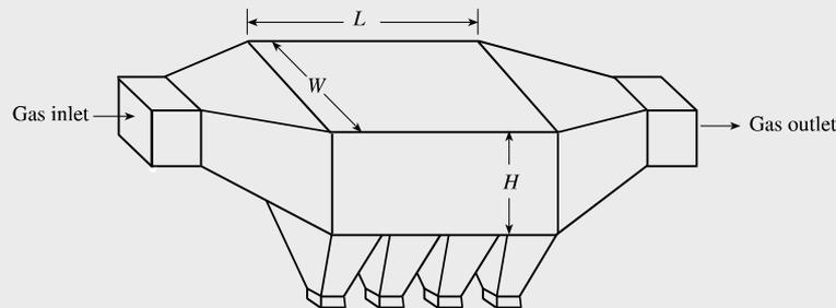
Spherical dust particles having a density of  $2200 \text{ kg/m}^3$  are to be separated from an air stream at a temperature of  $25^\circ\text{C}$ . Determine the diameter of the smallest particle that can be removed in a settling chamber 7 m long, 2 m wide, and 1 m high.
