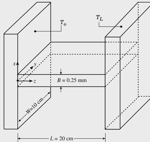
One of your friends assumes that there is no internal generation of energy within the fin and determines the steady-state temperature distribution within the fin as
