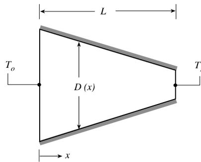
**Figure 1.2.** Heat transfer through a solid circular cone.
