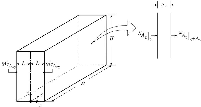
Figure 10.7. Mass transfer into a rectangular slab.
