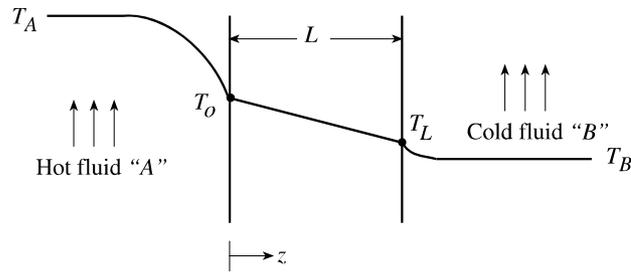
Figure 8.14. Heat transfer through a plane wall.
