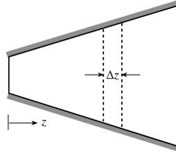
Figure 8.5. Conduction through a slightly tapered slab.
