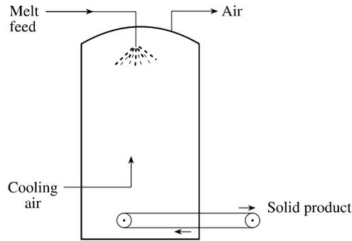
Figure 7.3. Schematic diagram of a spray cooling tower.
