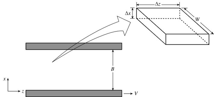
Figure 8.1. Couette flow between two parallel plates.
