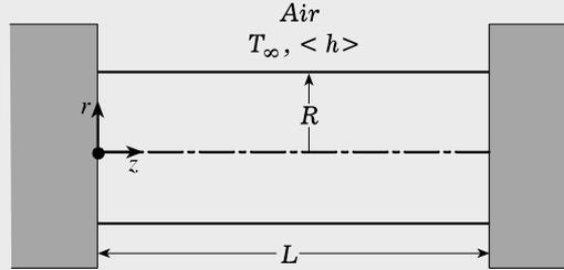
a) Consider a cylindrical differential element of thickness  $\Delta r$  and length  $\Delta z$  within the rod and show that the conservation statement for energy leads to
