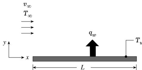
Figure 3.3. Flow over a flat plate.
