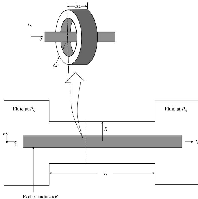
Figure 8.3. Couette flow in a concentric annulus.
