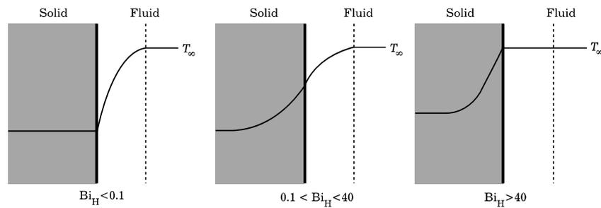
Figure 10.2. Effect of  $Bi_H$  on the temperature distribution.
