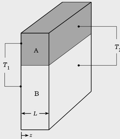
Figure 8.11. Composite plane wall in parallel arrangement.
