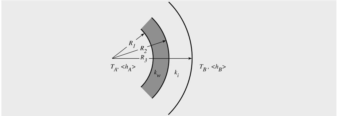
Figure 8.24. Conduction through an insulated hollow sphere.
