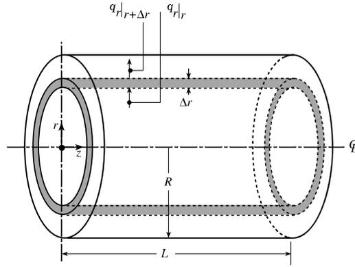
Figure 11.3. Unsteady-state conduction in a cylinder with generation.
