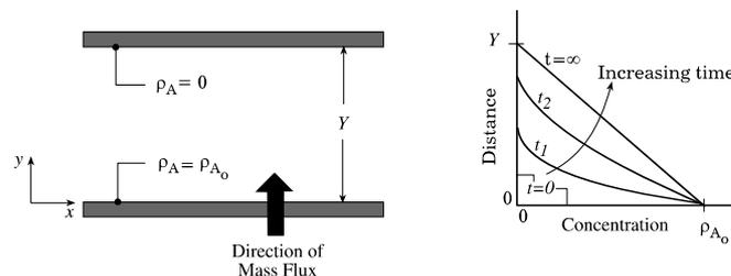
**Figure 2.4.** Concentration profile development between parallel plates.
