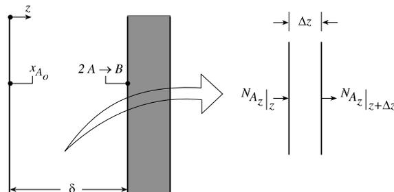
Figure 8.40. Heterogeneous reaction on a catalyst surface.
