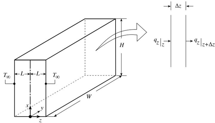
Figure 10.3. Unsteady-state conduction through a rectangular slab.
