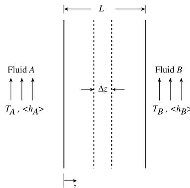
Figure 9.5. Conduction through a plane wall with generation.
