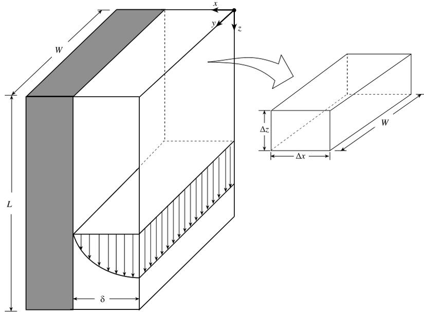
Figure 9.2. Falling film on a vertical plate.
