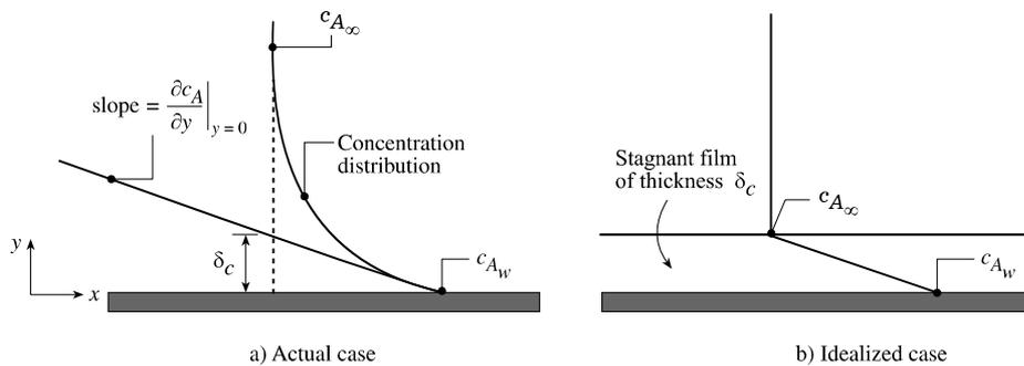
**Figure 3.6.** The film model for mass transfer.
