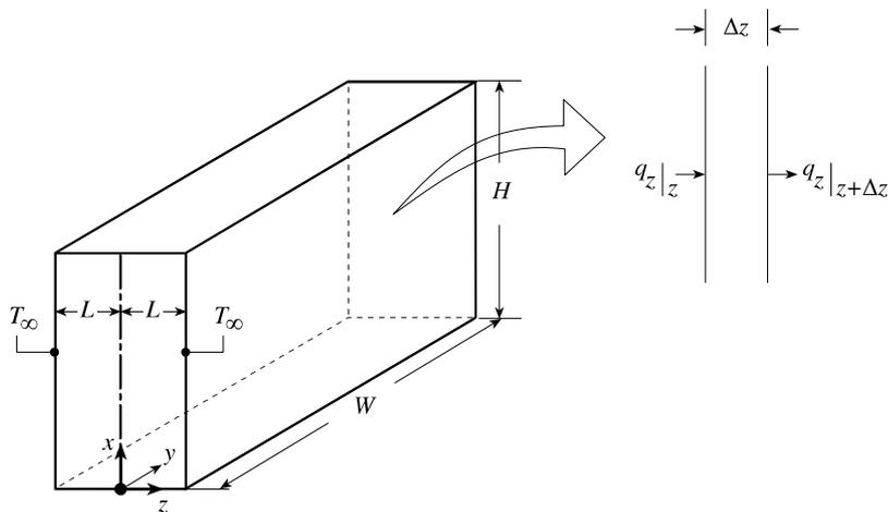
Figure 11.2. Unsteady-state conduction in a slab with generation.
