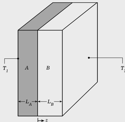
Figure 8.9. Composite plane wall in series arrangement.
