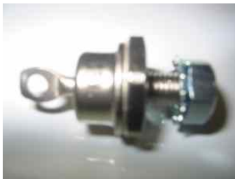
Optional: For higher amperages you can use High power diodes or rectifiers. 40 amp x 600 v
