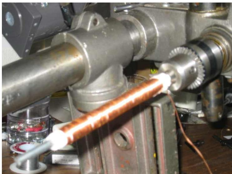
Small Drill press turned into a Coil Winder. We turned this by hand.
