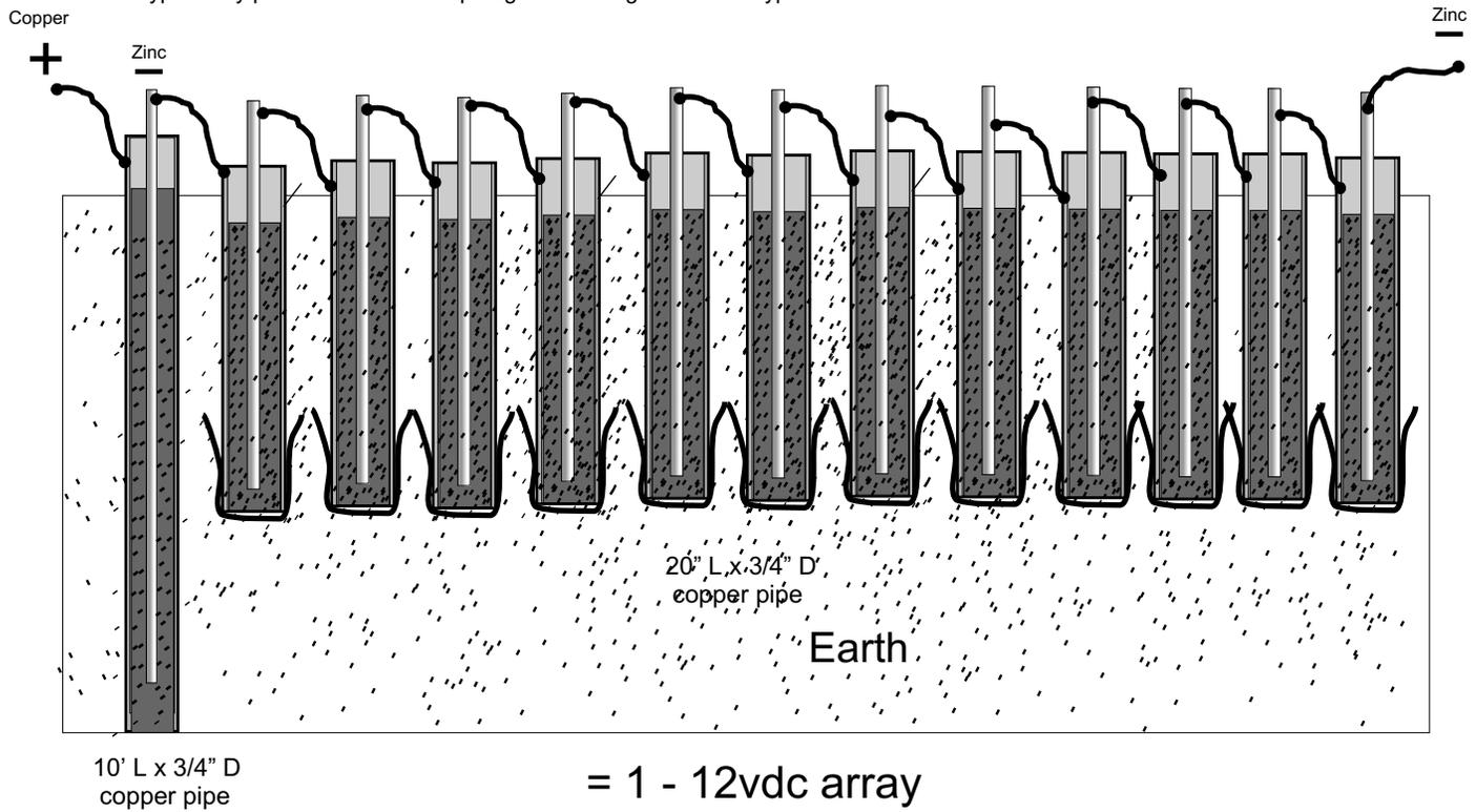
NOTICE: Do not paint the 10 foot copper cell. Keep all copper exposed to the earth. The more exposed copper the better. For higher amperage output, use a zinc or aluminum rod 10/16" Diameter which will leave a space of more than 1/16" to the copper.
