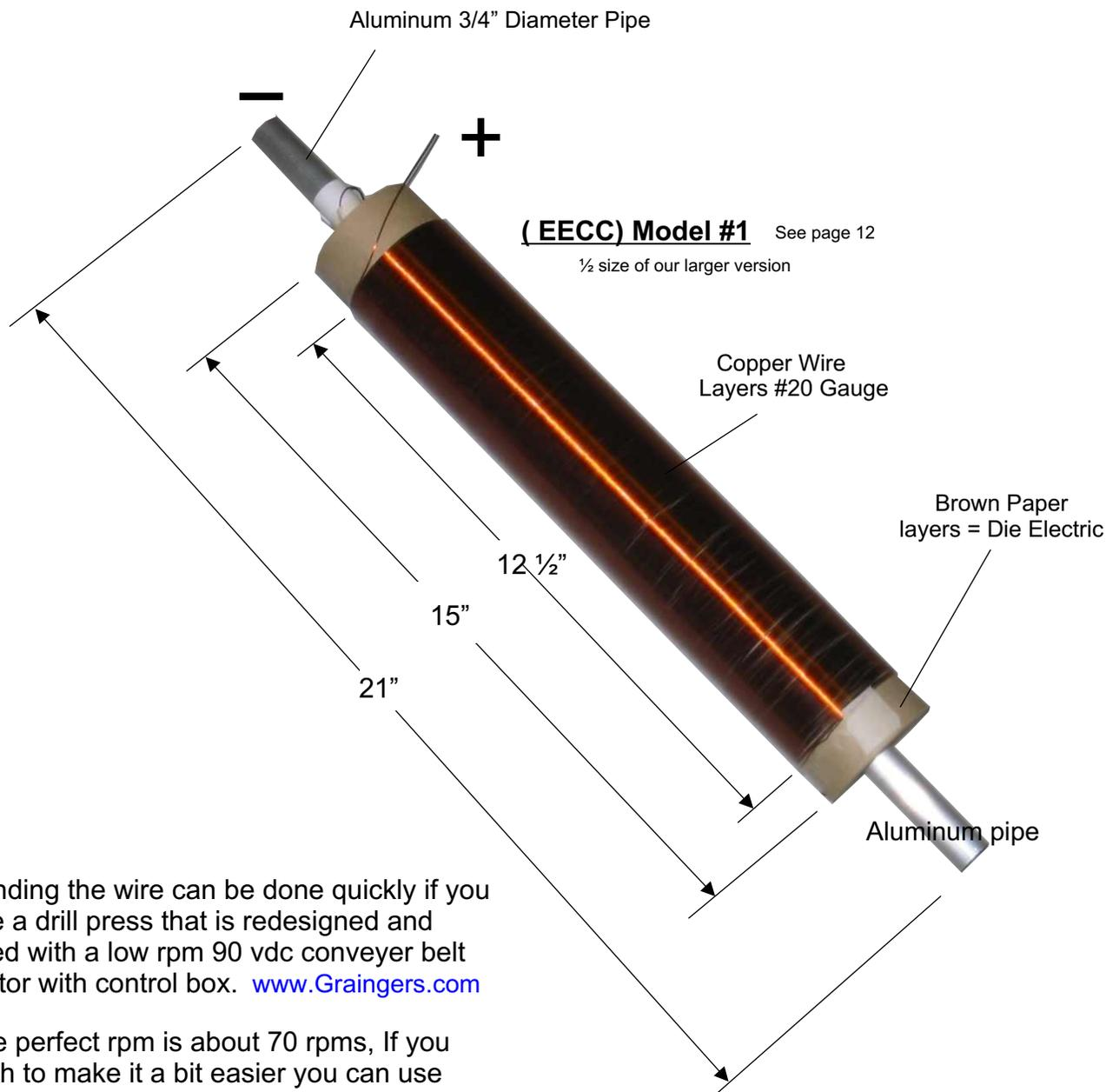
Winding the wire can be done quickly if you use a drill press that is redesigned and fitted with a low rpm 90 vdc conveyer belt motor with control box. [www.Graingers.com](http://www.Graingers.com)
