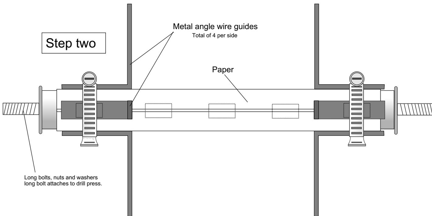
Apply first layer of wire, remove, metal wire guides, apply more paper, then repeat over and over again until you have about a 5 to 6 inch diameter roll of wire and paper. Makes a very powerful earth capacitor!
