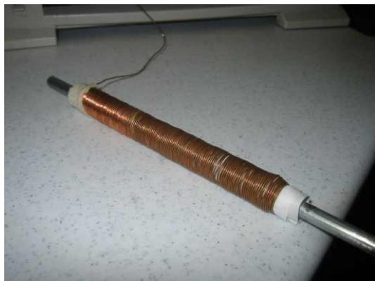
Our small test model #1, we used #22 bare copper wire wrapped around a zinc rod, each layer had a paper die electric, tested in tap water. 5 layers.
