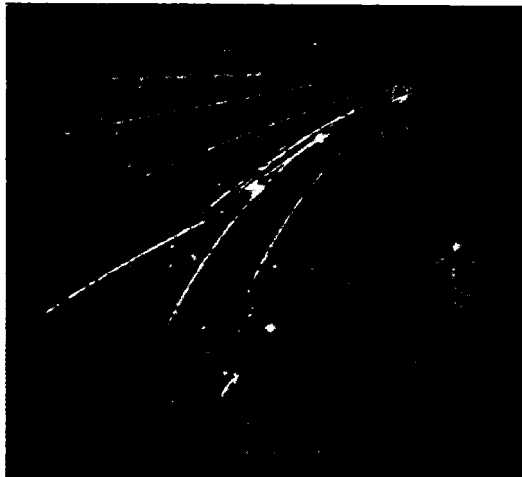
Fig. 11. Cosmic ray shower. Nineteen tracks diverging nearly horizontally from a point to one side of the chamber ( H = 14,000 gauss). Total energy of visible particles is 5 \times 10^9 eV. Some of the individual particles have an energy of over 10^9 eV (1935).
