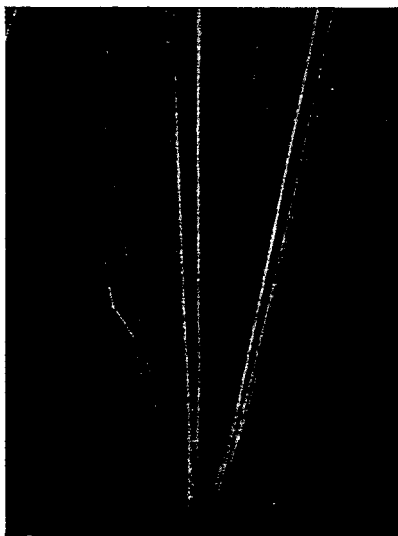
Fig. 4. Transmutation of nitrogen. One of the first photographs showing the capture of an alpha particle by a nitrogen nucleus with emission of a proton. The thin track moving to the right is the proton, and the short thick track to the left is due to the newly created ^{17}\text{O} nucleus. The alpha rays are from Thorium B + C (1925).
