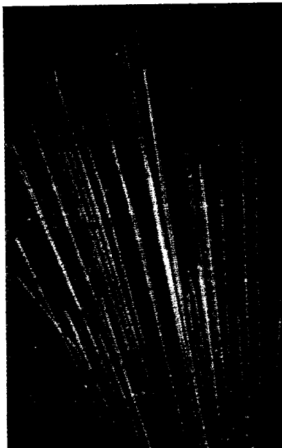
Fig. 2. Elastic collision of alpha particle with a hydrogen nucleus.
