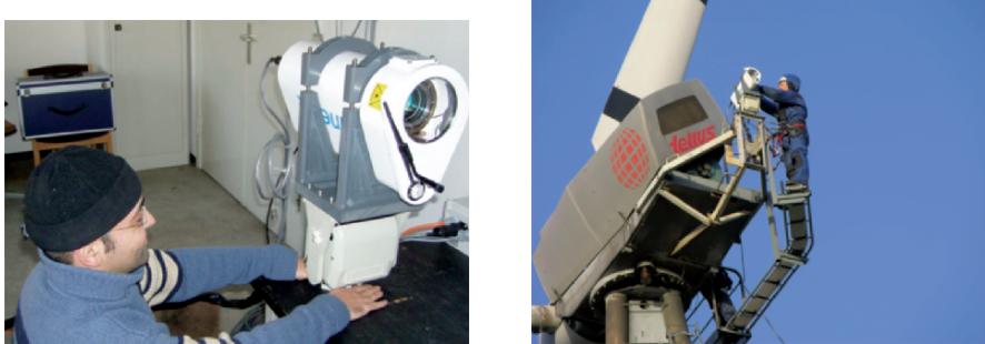
Fig. 15.4. Left: The telescope head of the laser Doppler anemometer from QinetiQ [9]. Right: Mounting of the laser anemometer behind the nacelle of a Tellus turbine
