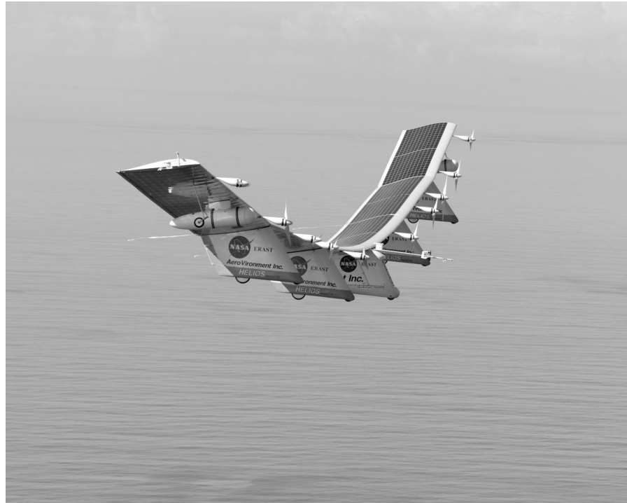
Figure 29.1. NASA's Helios prototype electrically powered flying wing. Image Credit: NASA Dryden flight research center, photo by Carla Thomas.
