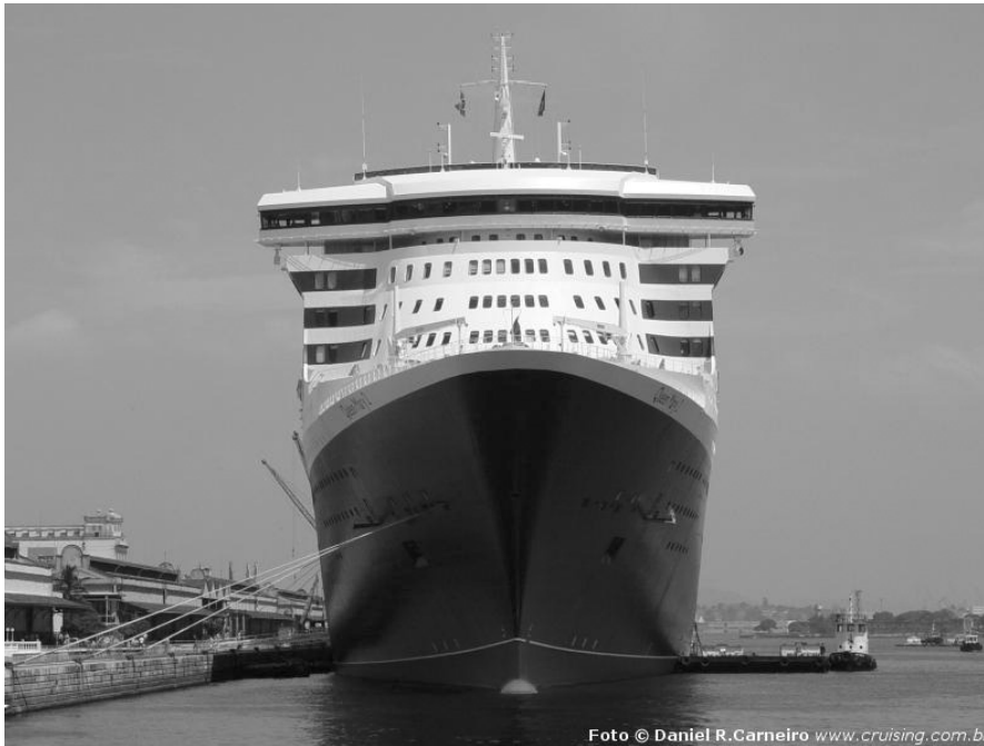
Figure 5.2. The Queen Mary 2 set sail on its maiden voyage on January 2, 2004. It is the world's largest ocean liner—ever—with a length of 345 m, a height of 72 m from keel to funnel, and a width of 41 m. Having a draft of only 10 m, its superstructure rises an impressive 62 m over the waterline. The low average density of the superstructure, including 2620 passengers and 1253 crew, combined with the high average density of the 117 megawatt engines and other heavy facilities close to the bottom of the ship nevertheless allow the stability condition to be fulfilled. Photograph by Daniel Carneiro.
