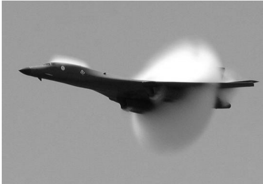
Figure 29.5. Prandtl–Glauert condensation around a B1 bomber passing the sound barrier. Crossing the Prandtl–Glauert ‘singularity’ at Mach 1, the pressure drops sharply and creates this condensation cloud in humid air. Photograph by Gregg Stansbery.
