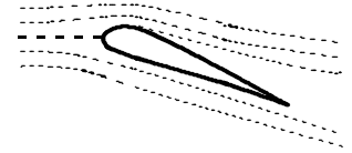
Sketch of the flow around an airfoil at large angle of attack. The boundary layer separates near the leading edge and replaces the previously laminar flow above the wing with turbulent flow yielding small lift and large drag.
