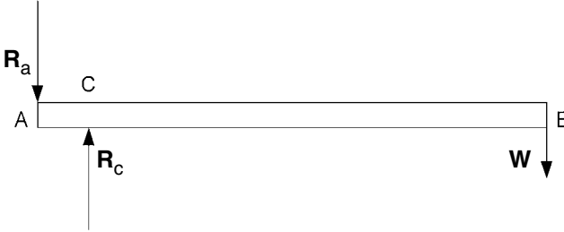
Figure 2.33. Forces acting on a cantilever beam.
