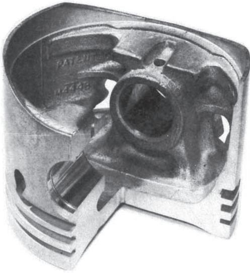
Fig. 3.4 In the Hepolite W-slot piston there is one slot in each face. It extends along the base of the oil control ring groove and, as shown in this illustration, its ends are swept round the gudgeon pin bosses
