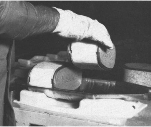
Fig. 14.4 Two monolithic catalyst carriers being assembled in series into their casing in the AC-Delco factory at Southampton
