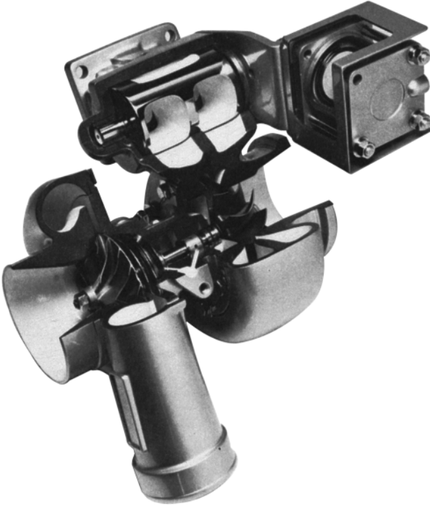
Fig. 8.12 A pneumatically controlled exhaust brake, top, integral with the turbocharger is an option
