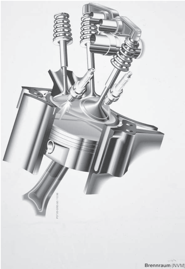
Fig. 4.20 With three valves per cylinder, it is easy to accommodate two sparking plugs
