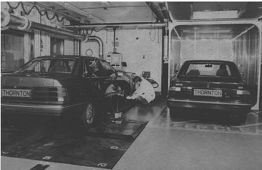
Fig. 14.6 ( Left ) Sealed Housing for Evaporative Determination (SHED) installed alongside a chassis dynamometer ( right ) in a thermostatically controlled chamber at the Shell Thornton Research laboratories
