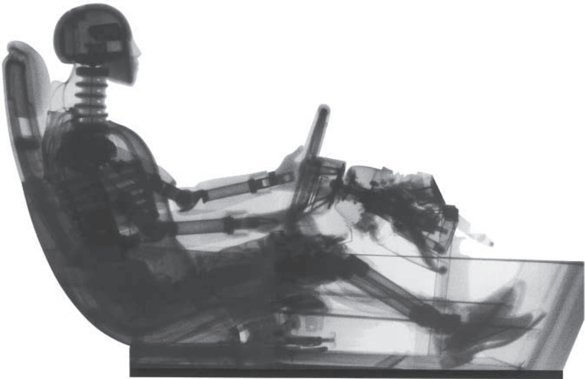
Fig. 36.1 MIRA has developed a method of X-ray imaging of tests at a rate of 1000 frames per second, which enables them to view regions which conventional cameras cannot access, for example around the pedals
