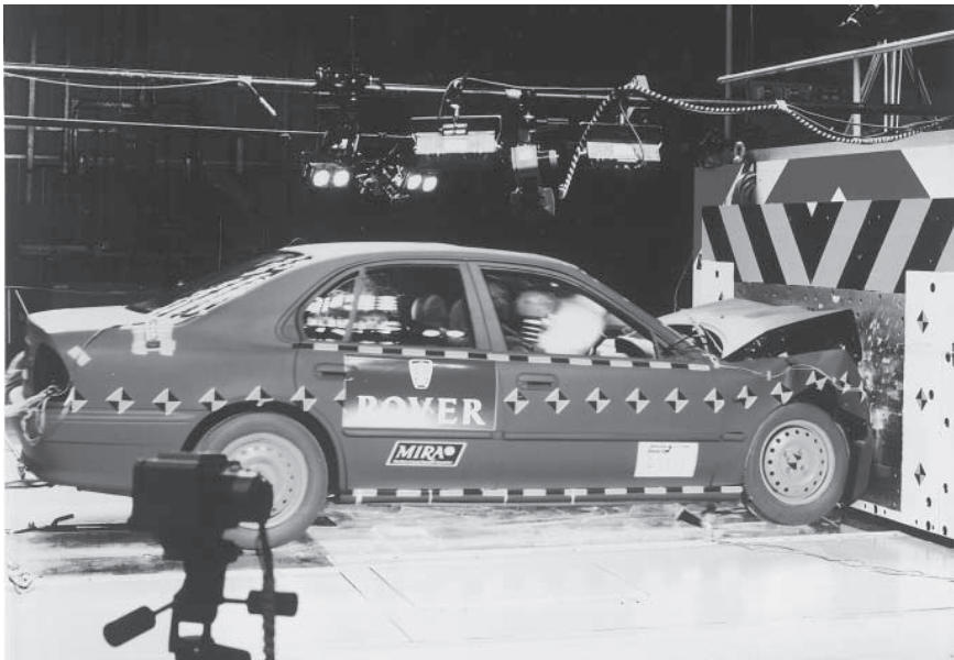
Fig. 36.2 For conventional frontal impact tests, the impacted face of the concrete block can be protected with steel plate to reduce the rate of erosion
