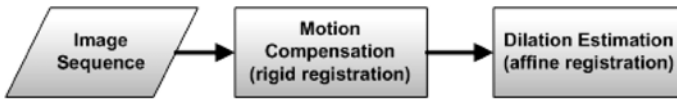
Figure 5.3: Overview of the proposed two-stage method: after motion compensation is carried out by recovering a rigid motion model, the vasodilation is measured by computing the scaling factor along the normal to the artery that best matches the two analyzed frames.
