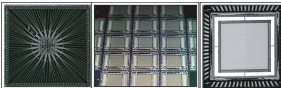
FIGURE 6.4. Shows Nanogen’s 100 test site microelectronic array, a silicon wafer of 400 test site microarrays and a packaged 10,000 test site microarray. The 400 and 10,000 test site arrays have CMOS electronic control elements incorporated into the chips underlying structure.
