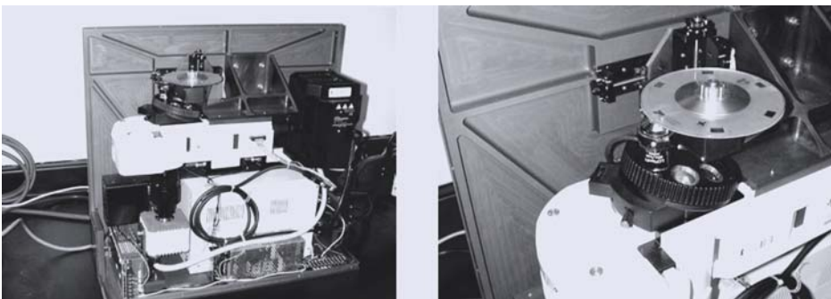
FIGURE 10.9. Left: Optical disc drive/imager with cover removed. Size of unit is made to fit in specific cargo bay of Space-Lab. Right: Zoom of microscope objectives and a disc loaded in the drive.
