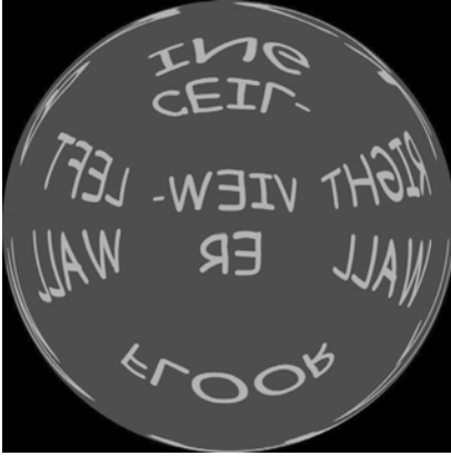
Figure V.10. An environment map mapped into a sphere projection. This is the kind of environment map supported by OpenGL. See Color Plate 7.
