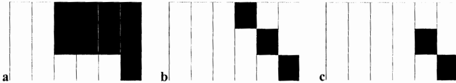
Figure 6.24. Hopfield net illustrating the probabilities associated with the assignments corresponding to the example shown in Figure 6.23. (a) Feasible assignments as solutions to the quadratic problem; (b) A candidate assignment; (c) final assignment corresponding to the previous situation ( q=2 ).
