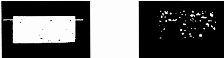
Figure A.1. Example of a cork stopper image at the left and the corresponding binary image of the defects at the right.
