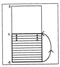
The situation where the elevator is at the bottom of the shaft and m falls is similar to the case where the elevator is not at the top or bottom of the shaft. It simply moves up by dm.
