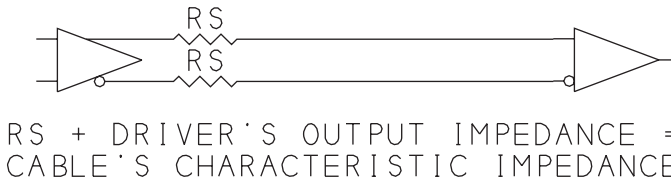
Figure 7-7: A series termination can absorb reflections.
